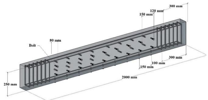
Figure 2. Side 1 and bottom bolts 3D design
