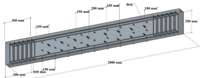
Figure 3. Side 2 and bottom bolts 3D design
