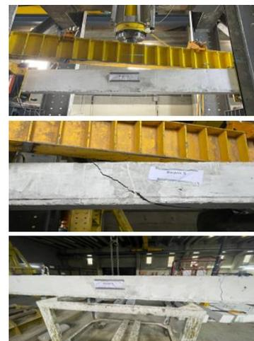
**Figure 14.** Beam B5 mode of failure
