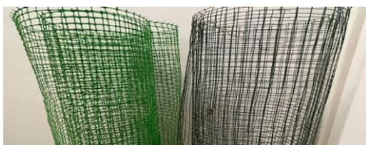
Figure 1. Plastic and steel chicken wire
