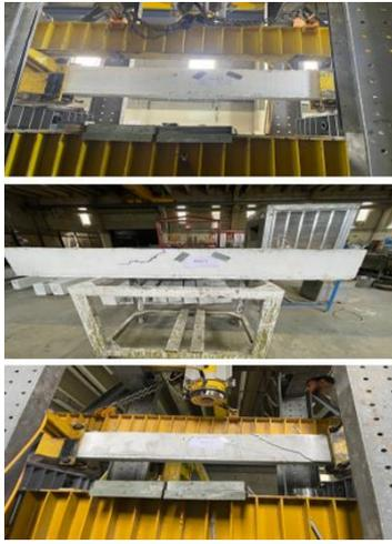
**Figure 15.** Beam B6 mode of failure
