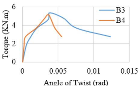
**Figure 6.** B3, B4 torque twist curve
