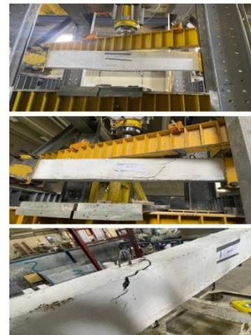
**Figure 12.** Beam B3 mode of failure
