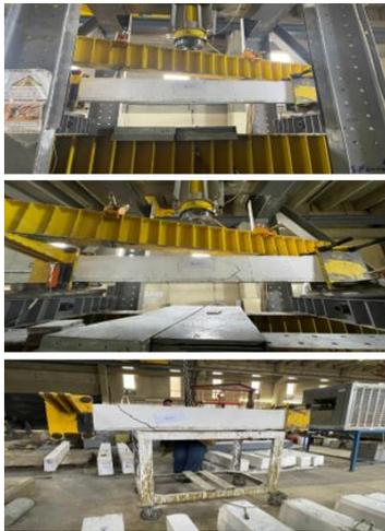
**Figure 16.** Beam B7 mode of failure
