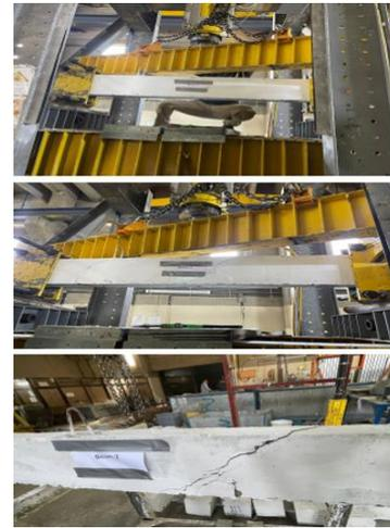
**Figure 11.** Beam B2 mode of failure
