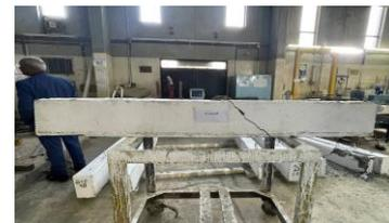
**Figure 13.** Beam B4 mode of failure
