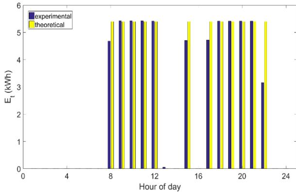
**Figure 5.** Comparison between the thermal energy produced by the electric heater and that resulting from the optimization tool
