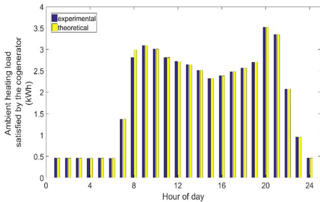
**Figure 6.** Comparison between the experimental and theoretical SH load satisfied by the CHP
