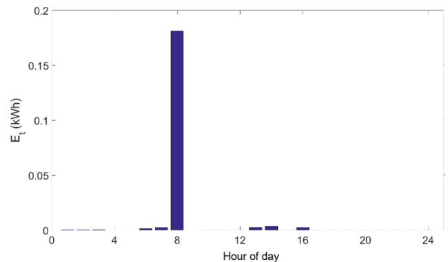
**Figure 8.** Thermal load satisfied by the auxiliary boiler in the experimental case
