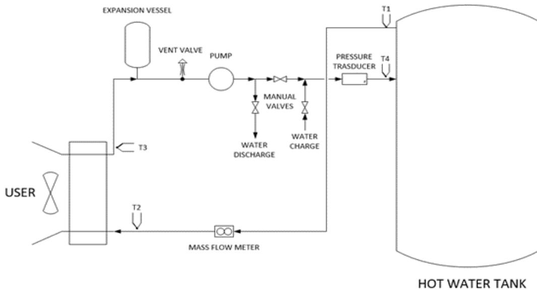
Figure 4. Scheme of the user circuit
