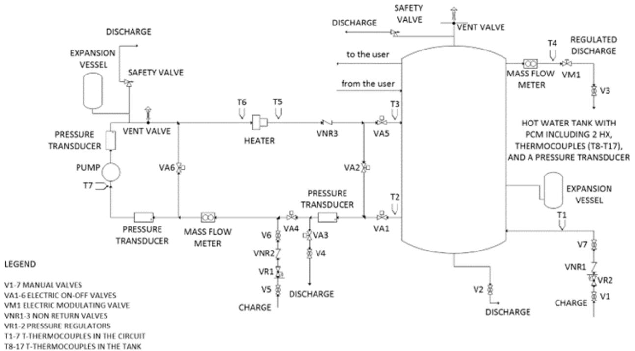
Figure 3. Scheme of the heat generator circuit
