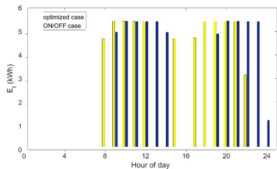
**Figure 9.** Comparison between the thermal energy produced by the electric heater with ON/OFF and that resulting from the optimization tool
