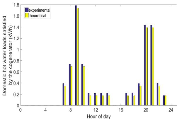
**Figure 7.** Comparison between the experimental and theoretical DHW consumption satisfied by the CHP
