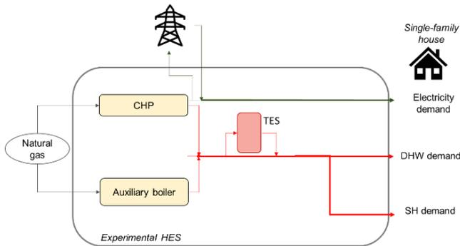
**Figure 1.** Scheme of the experimental HES for the operation optimization model
