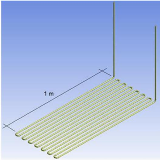
**Figure 1.** Horizontal ground heat exchanger
