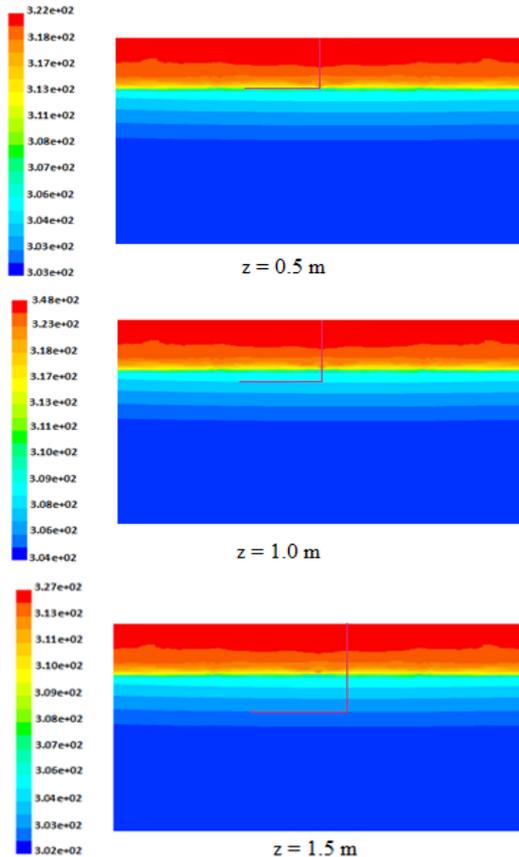
**Figure 4.** Contours of temperature distribution for the soil pile at 12:00 PM
