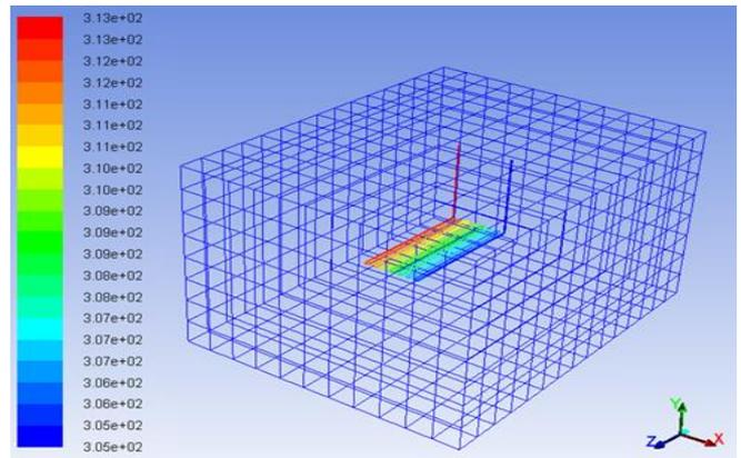
**Figure 5.** Contours of temperature distribution for the pipe loops, water mass flow rate equal to 0.0278 kg/s, in a 1.0 m depth, at 12:00 PM
