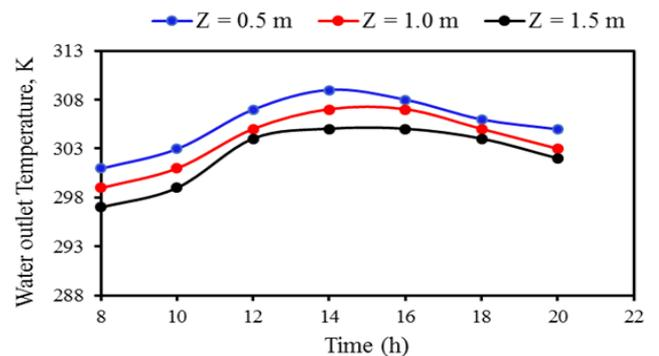
**Figure 6.** Water outlet temperature as a function of time of the day for different depths, on 11 July
