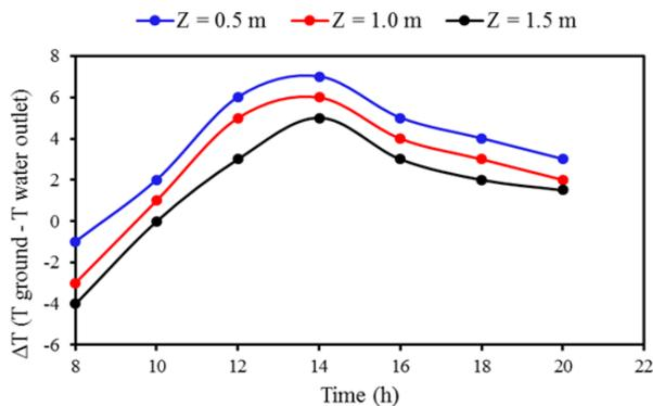
**Figure 7.** Temperature difference between the ground and the output water on 11 July
