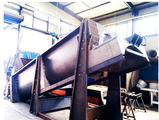
Figure 8. Mechanical parts of carpentry of the drier prototype auger
