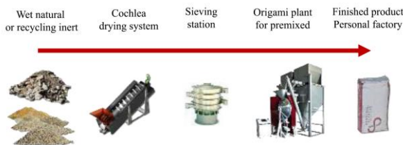
Figure 3. Production process from wet to dry premix finished inert.
