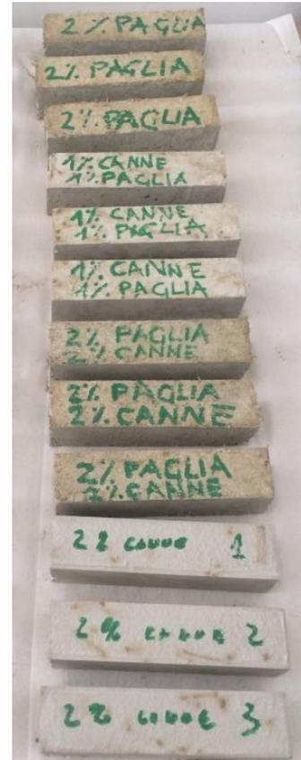
**Figure 6.** Specimens for mechanical strength tests
