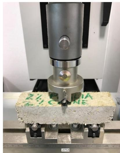
**Figure 8.** Three point flexural test on 2C2P specimen
