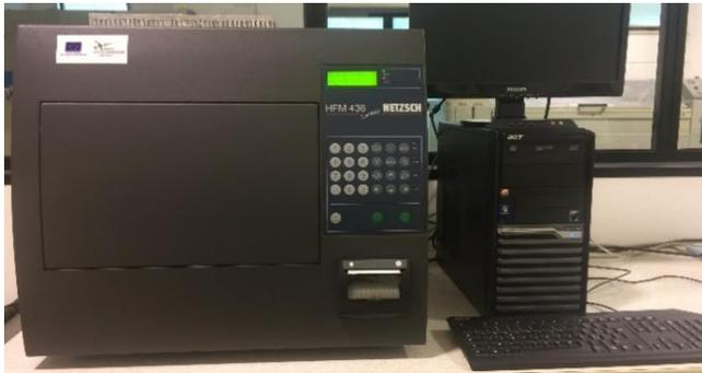
**Figure 7.** NETZSCH heat flow meter HFM 436/0/1
