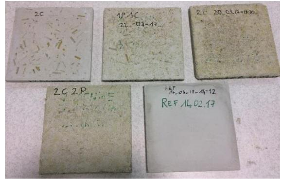
**Figure 5.** Specimens for thermal conductivity tests
