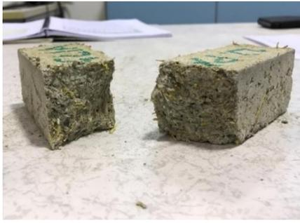
**Figure 9.** Section after breaking of 2P specimen
