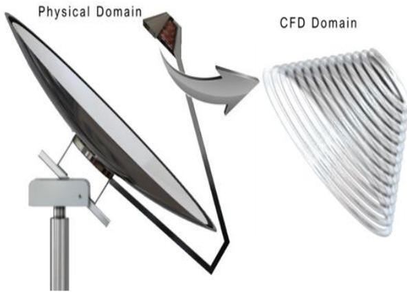
**Figure 1.** A solar dish system, the physical and CFD domains
