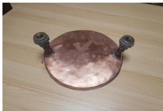
**Figure 10.** The reference circular solar receiver
