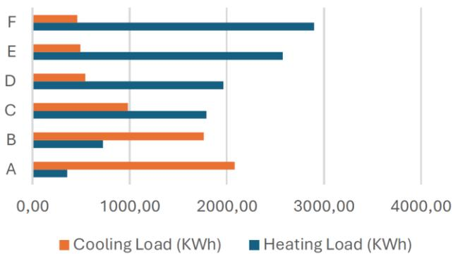
**Figure 9.** Average heating and cooling load by climate category
