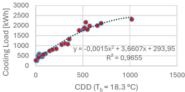
**Figure 8.** Correlation analysis: Cooling load and CDD18
