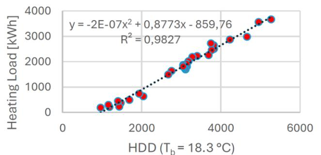
**Figure 7.** Correlation analysis: Heating load and HDD18
