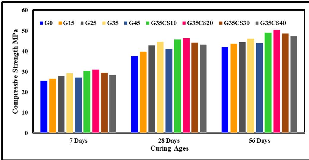
Figure 2. CS of sustainable concrete using GGBS and CLS
