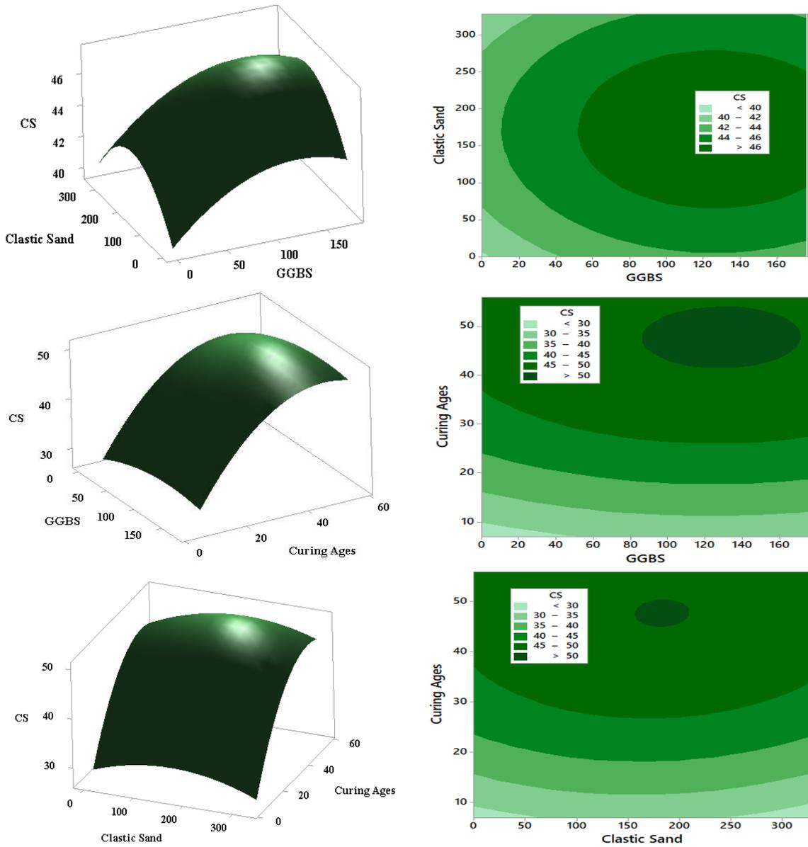
**Figure 7.** Response surface and contour plots for “GGBS”, “CLS”, “Curing Ages” Vs mean CS
