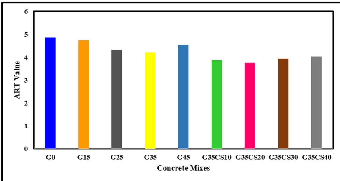
Figure 5. Absorption resistance test of sustainable concrete using GGBS and CLS
