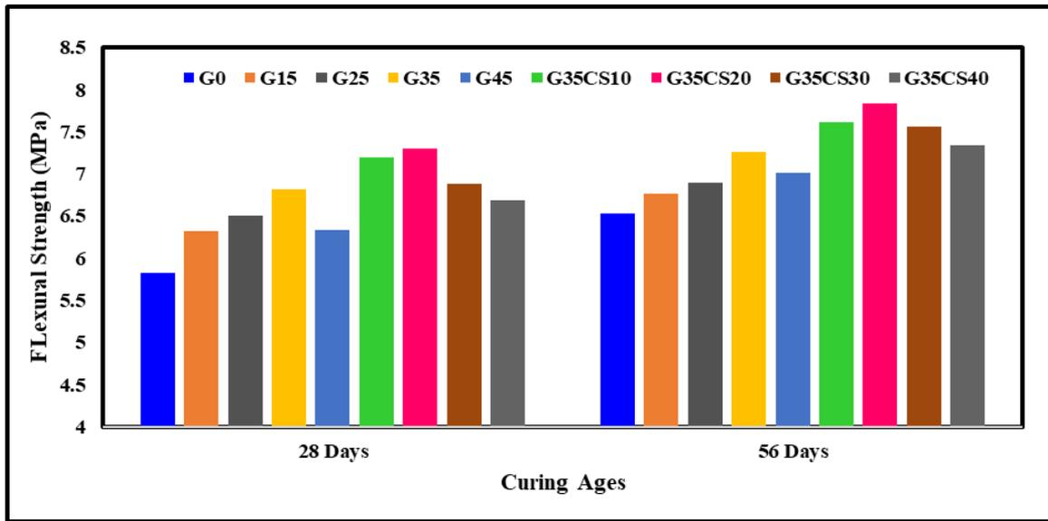
Figure 4. Flexural strength of sustainable concrete using GGBS and CLS
