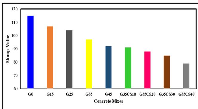
**Figure 1.** Slump flow values
