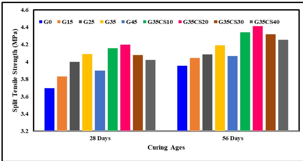
Figure 3. SPT of sustainable concrete using GGBS and CLS
