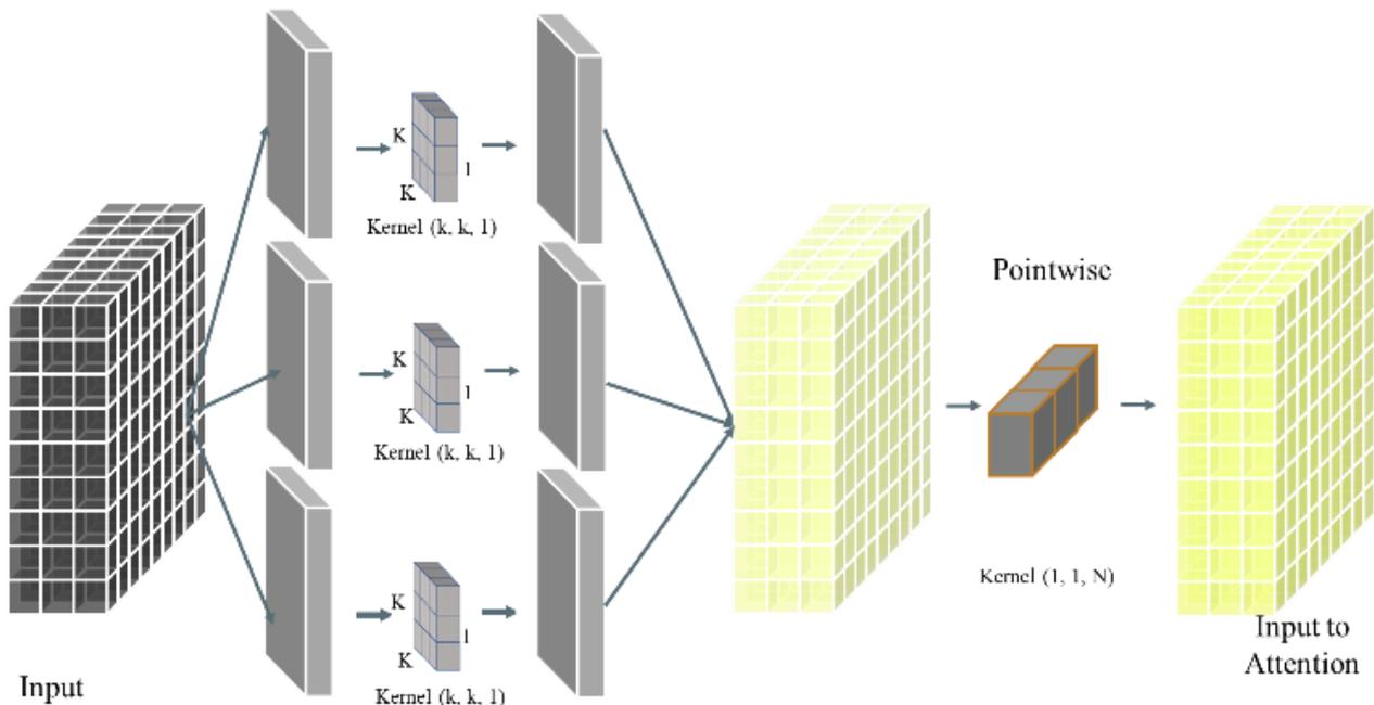
Figure 2. 1D CNN depthwise separable architecture
