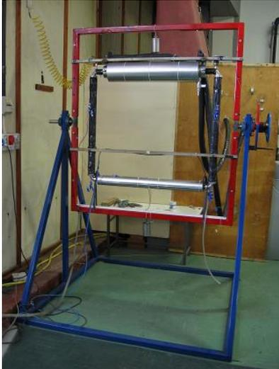
**Figure 1.** Experimental natural circulation loop [9]
