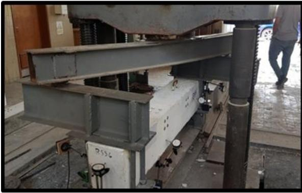
Figure 8. Beam tested by subsection to torsional moments
