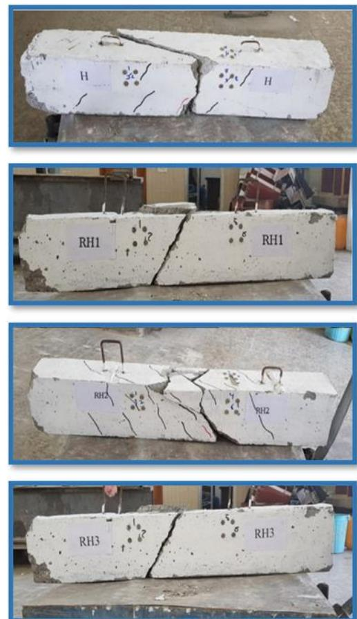
**Figure 5.** Failure mode of beams (mode "A")
