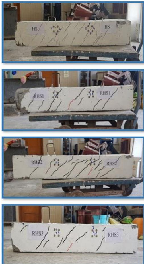
Figure 7. Failure mode of beams (mode “C”)
