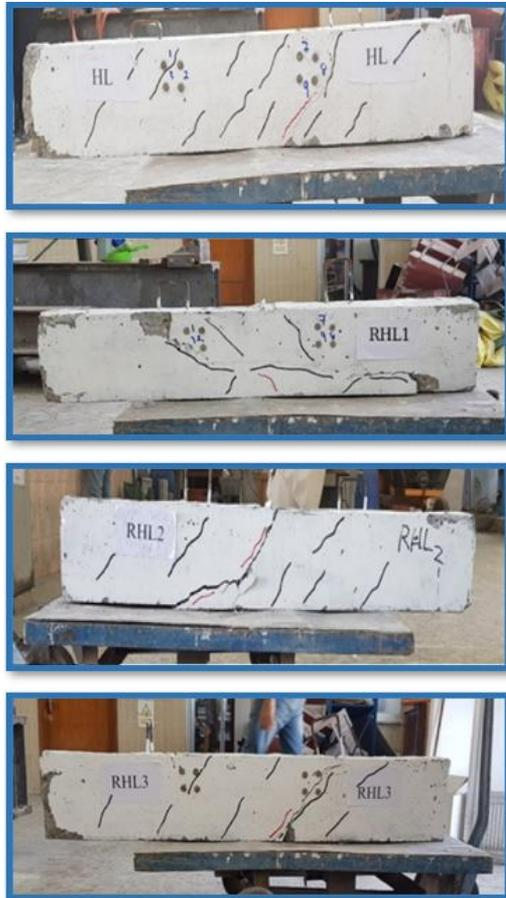
Figure 6. Failure mode of beams (mode “B”)
