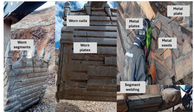
Figure 2. Excavator bucket wear and reinforcement
