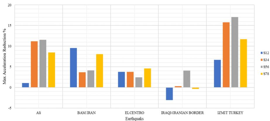
Figure 32. CFD located in two stories for different earthquakes
