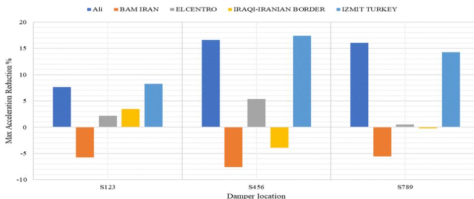
Figure 29. DFD located in two stories for different damper location
