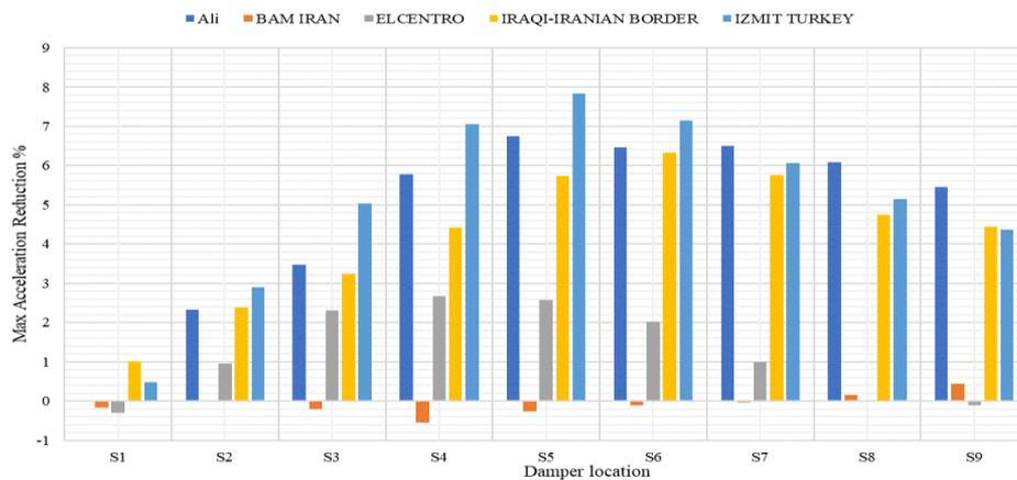
Figure 25. DFD located in one story for different damper location
