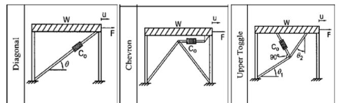
Figure 4. Damper friction configuration
