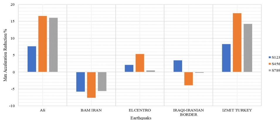
Figure 28. DFD located in two stories for different earthquakes
