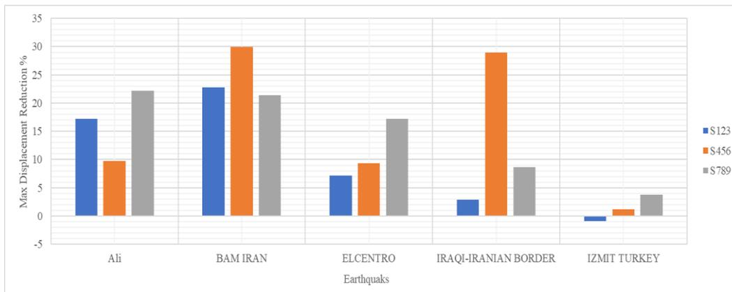
**Figure 10.** DFD located in three stories for different earthquakes
