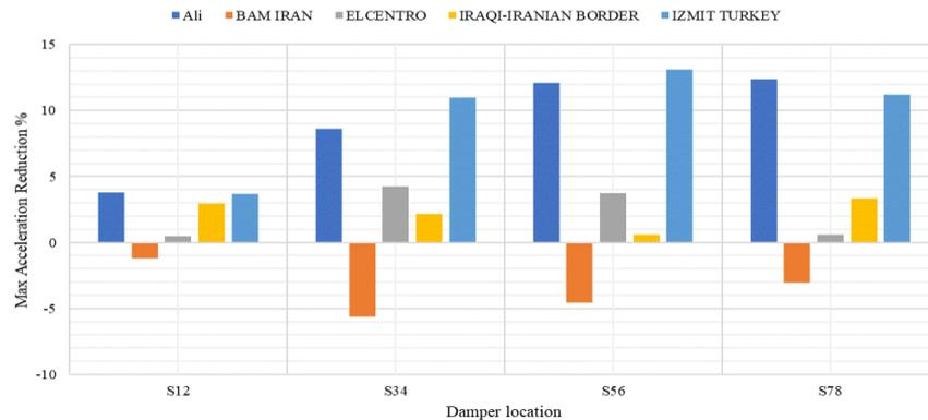
Figure 27. DFD located in two stories for different damper location
