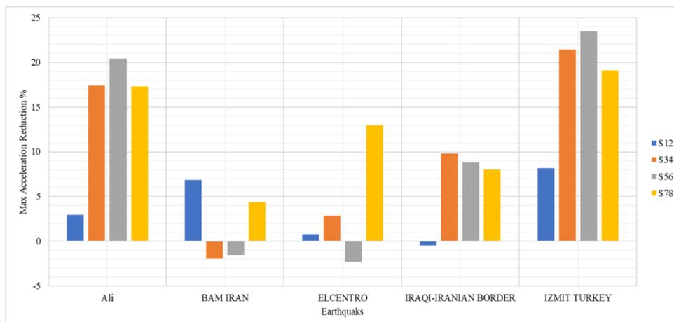
Figure 38. UTFD located in two stories for different earthquakes
