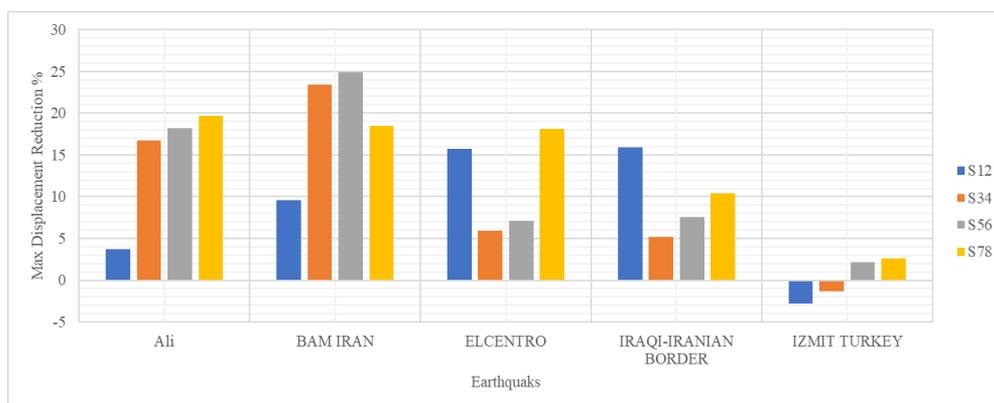
Figure 8. DFD located in two stories for different earthquakes
