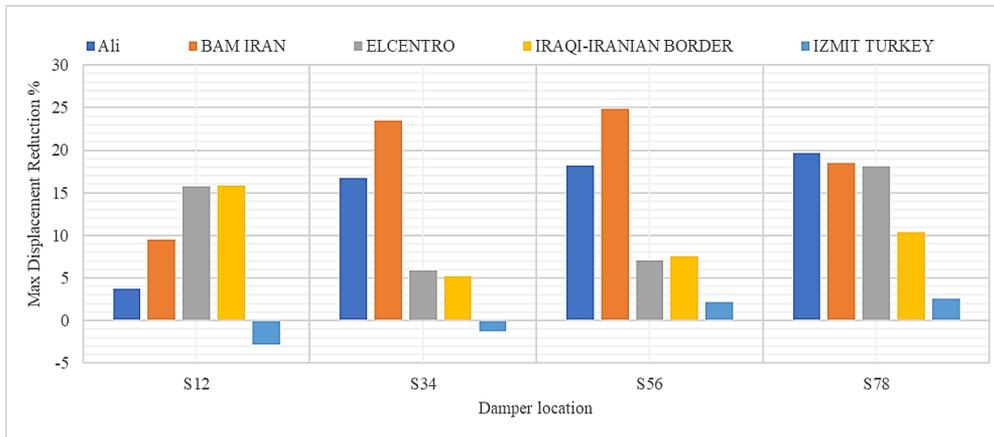
**Figure 9.** DFD located in two stories for different damper location
