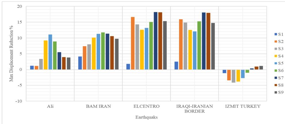
Figure 6. DFD located in one story for different earthquakes
