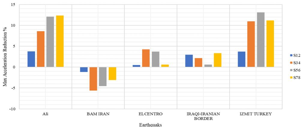
Figure 26. DFD located in two stories for different earthquakes
