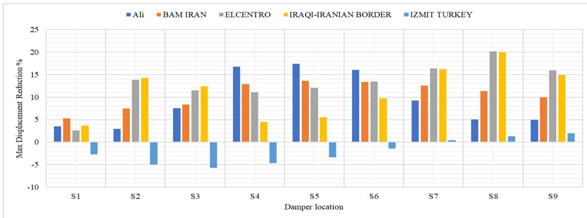
Figure 19. UTFD located in one story for different damper location
