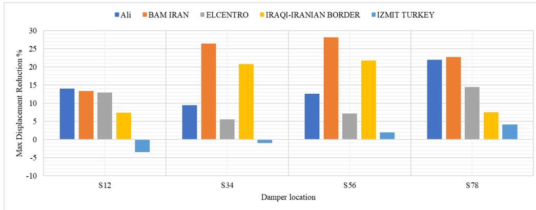
Figure 21. UTFD located in two stories for different damper location
