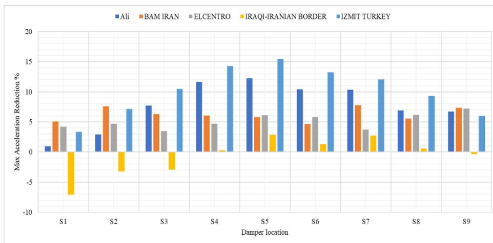
Figure 37. UTFD located in one story for different damper location
