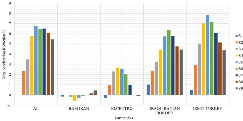
Figure 24. DFD located in one story for different earthquakes
