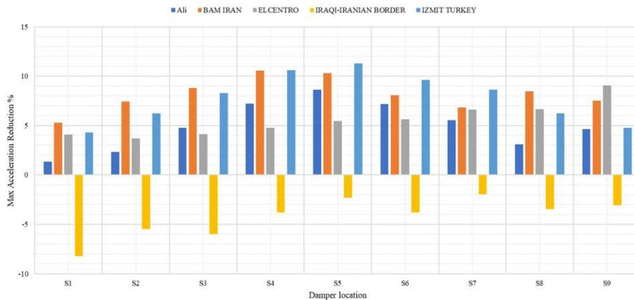
Figure 31. CFD located in one story for different damper location
