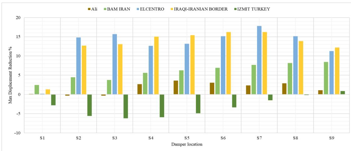
**Figure 13.** CFD located in one story for different damper location
