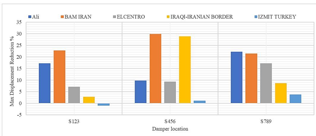
**Figure 11.** DFD located in three stories for different damper location
