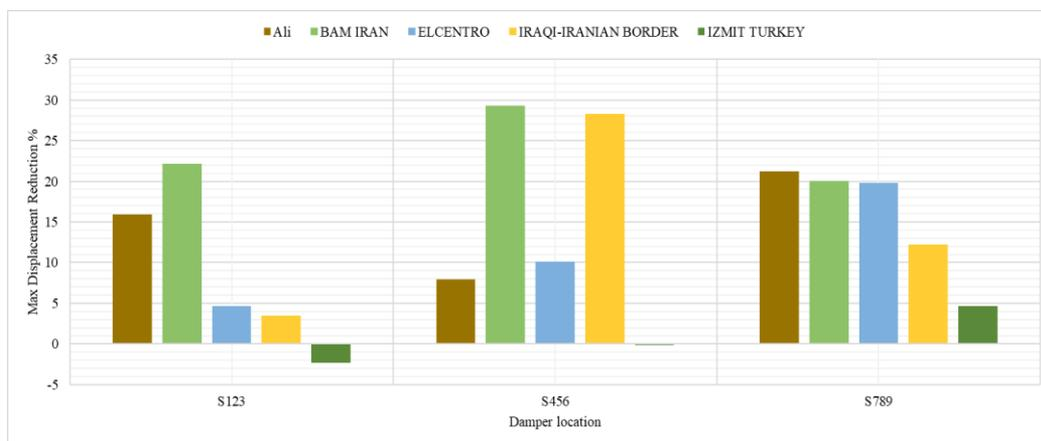
Figure 17. CFD located in three stories for different damper location
