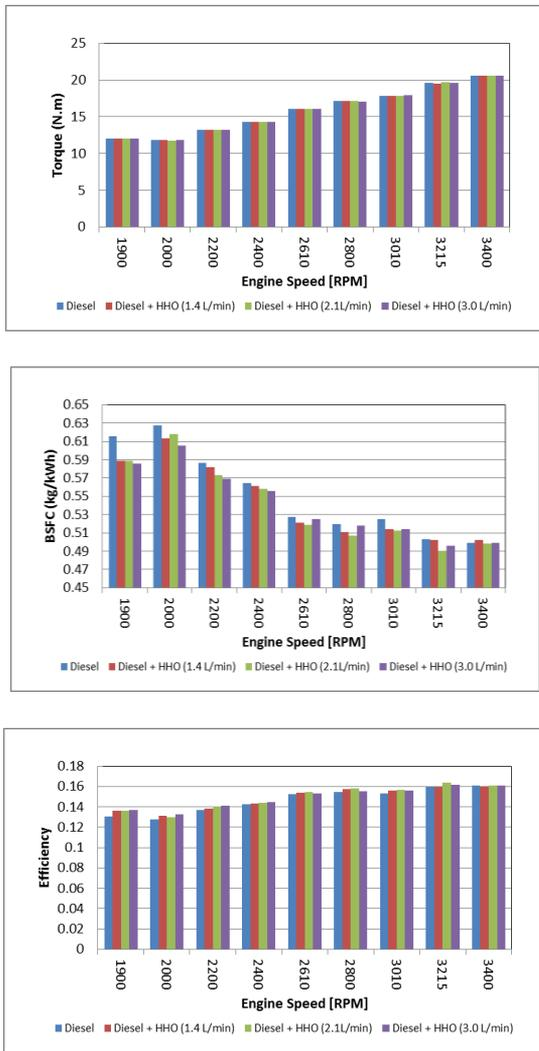
**Figure 6.** Power, torque, BSFC and efficiency as a function of engine speed (variable dynamometer speed)
