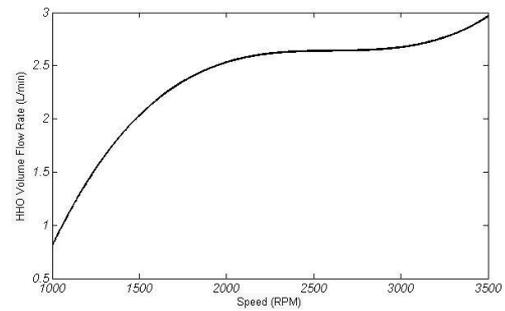
**Figure 7.** Power based optimum HHO flow rate at each speed
