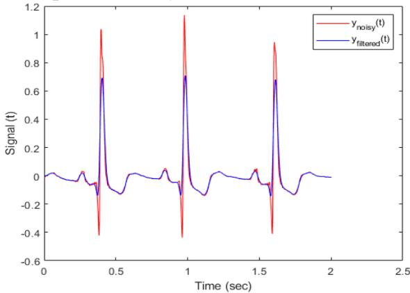
(d) Noisy ECG signal and equivalent filtered signal using the Gaussian filter (Parameter:  $\sigma=0.01$ )
