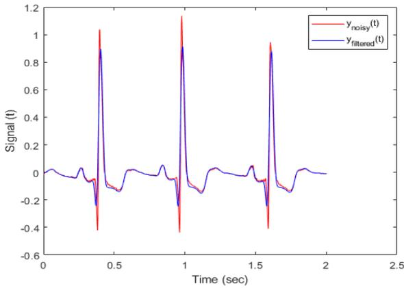
(c) Noisy ECG signal and corresponding filtered signal using the Mittag-Leffler filter (Parameters:  $\sigma=0.01$ ,  $\alpha=1.20$ , and  $\beta=1$ )
