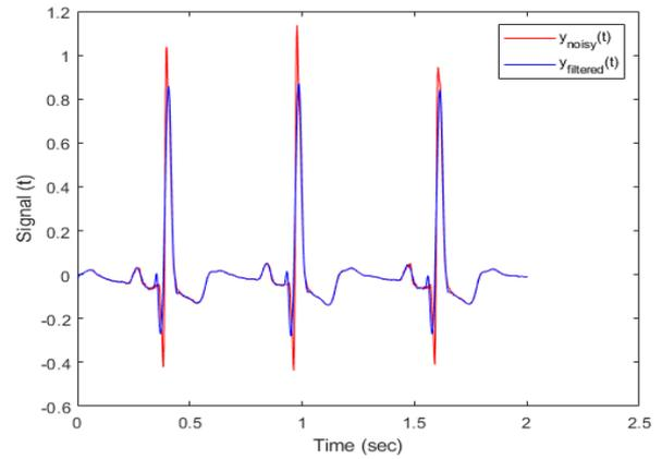
(g) Noisy ECG signal and equivalent filtered signal using the Savitzky-Golay smoothing filter (Parameters:  $nl=16$ ,  $nr=16$ ,  $M=4$ )
