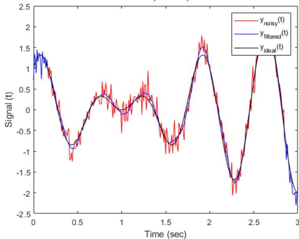
(f) Savitzky-Golay filtered signal vs. noisy and ideal signal with  $nl=16$ ,  $nr=16$ ,  $M=4$
