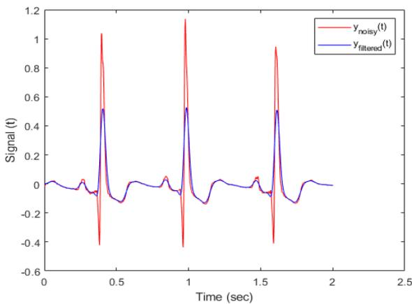
(e) Noisy ECG signal and equivalent filtered signal using the Gaussian filter (Parameter:  $\sigma=0.015$ )
