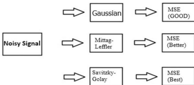
**Figure 3.** Block diagram representing the Gaussian filter, Mittag-Leffler filter, and Savitzky-Golay smoothing filter, with mean square error assessment
