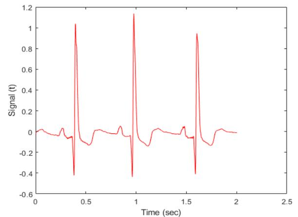
(a) Real ECG signal with noise within the timeframe of 0 to 2 seconds
