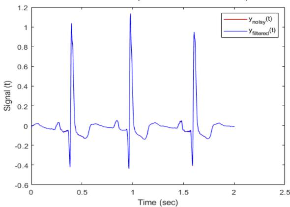
(f) Noisy ECG signal and equivalent filtered signal using the Savitzky-Golay smoothing filter (Parameters:  $nl=4$ ,  $nr=4$ ,  $M=4$ )
