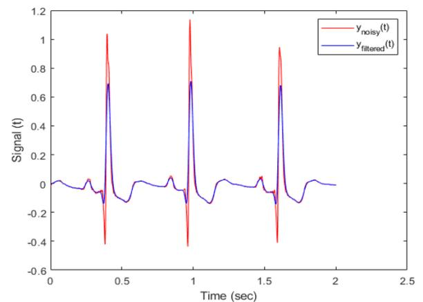
(b) Noisy ECG signal and equivalent filtered signal using the Gaussian variant of the Mittag-Leffler filter ( $\sigma=0.01$ ,  $\alpha=1$ , and  $\beta=1$ )
