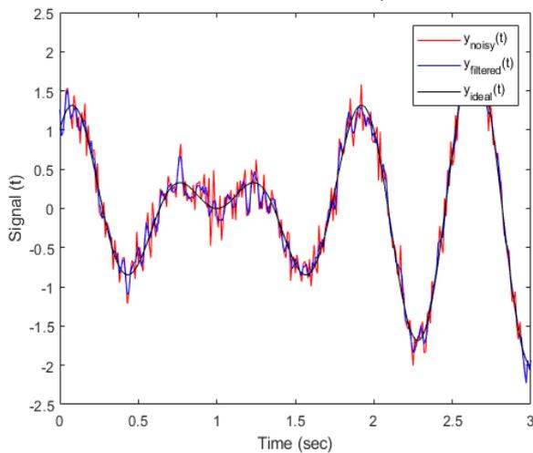
(e) Savitzky-Golay filtered signal vs. noisy and ideal signal with  $nl=4$ ,  $nr=4$ ,  $M=4$
