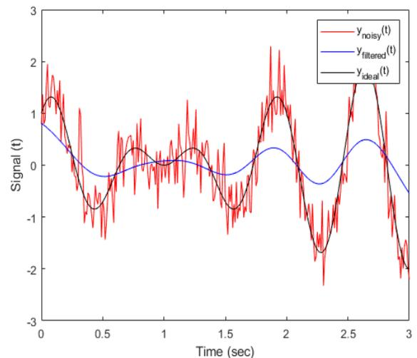
(c) Mittag-Leffler filtered signal vs. noisy and ideal signal with  $\sigma=0.2$ ,  $\alpha=1$ , and  $\beta=1$
