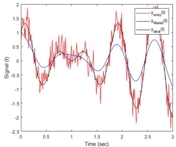
(b) Gaussian filtered signal vs. noisy and ideal signal with  $\sigma=0.15$
