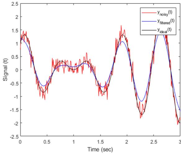
(d) Mittag-Leffler filtered signal vs. noisy and ideal signal with  $\sigma=0.1$ ,  $\alpha=0.95$ , and  $\beta=0.9$
