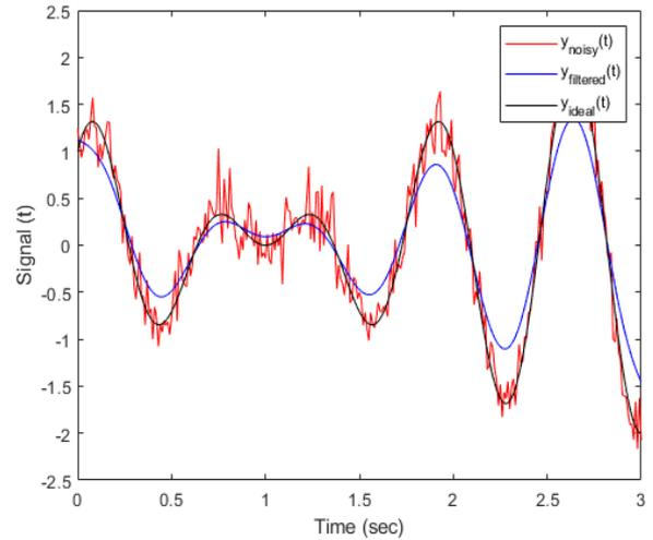
(a) Gaussian filtered signal vs. noisy and ideal signal with  $\sigma=0.1$
