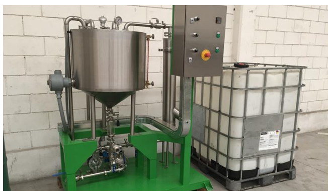
Figure 4. Biodiesel Plant MB-400, which yields up to 400 l/day of biodiesel
