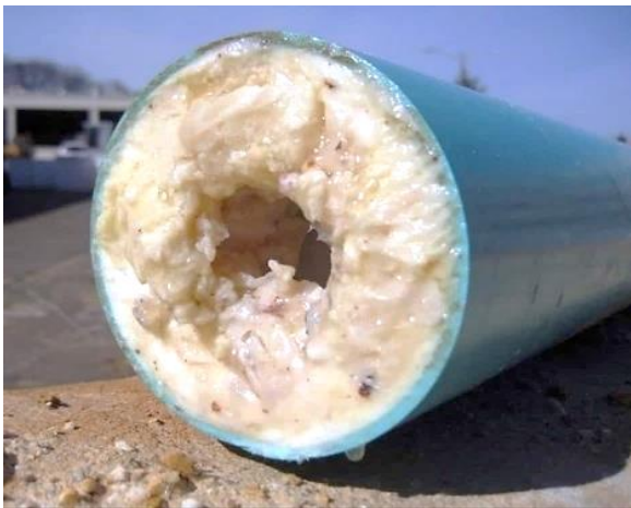
Figure 2. Sewer pipe clogged by excess solidified vegetable fats (supply canter Mexico City, Mexico) [26]
