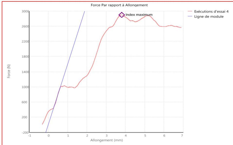
**Figure 3.** Simple compression test execution review graph
