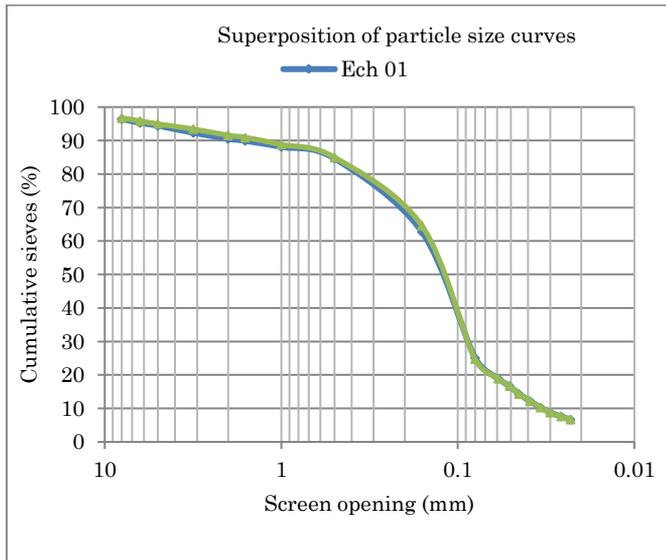
**Figure 1.** Superposition of the particle size curves of the 2 samples
