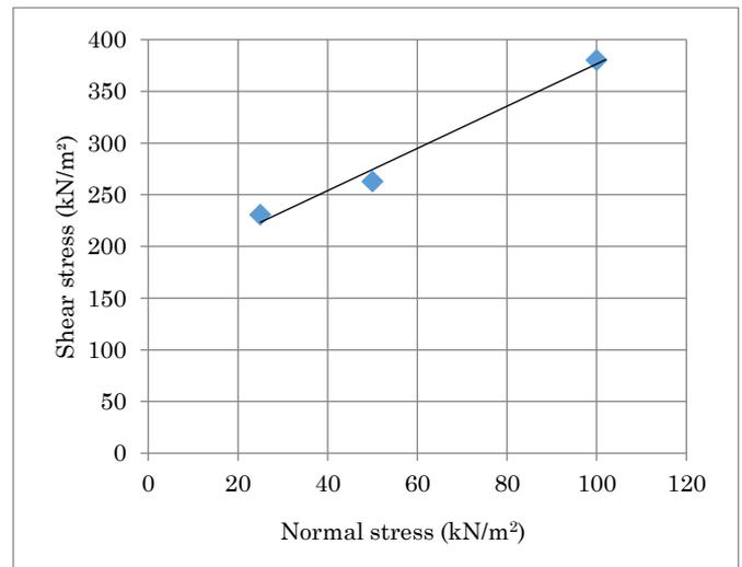
**Figure 2c.** Shear tests at constant normal stresses
