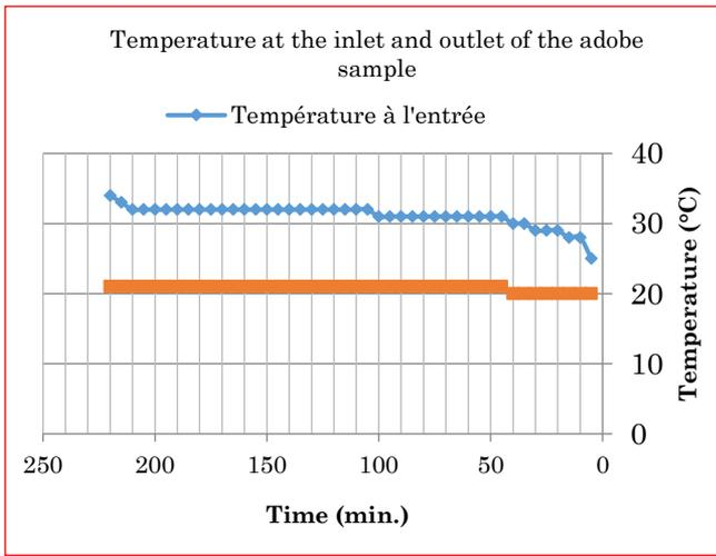
**Figure 4a.** Evolution of the temperature at the inlet and outlet of the adobe
