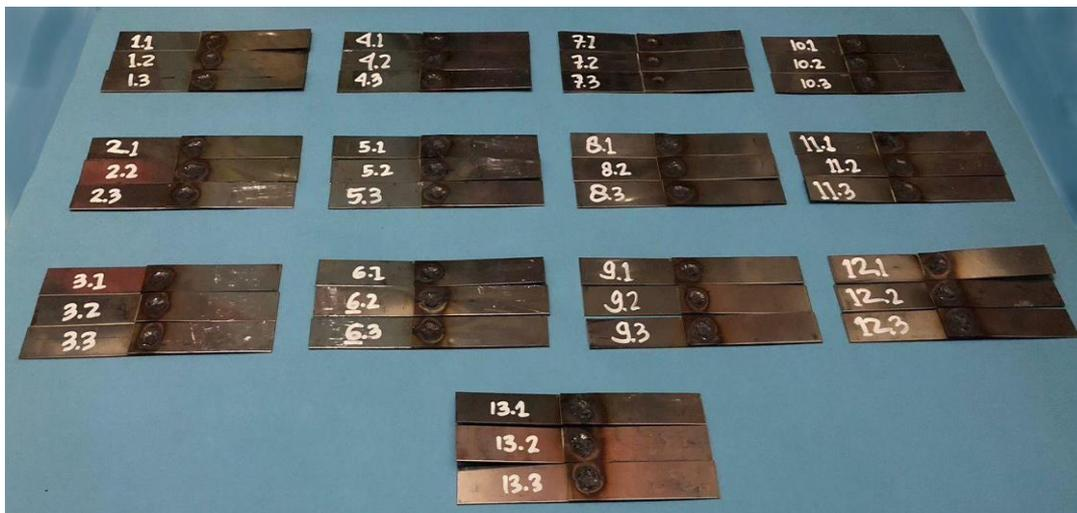
**Figure 3.** TIG welding coupon: 39-unit sample from 13 iterations of SUS 304 steel sheets
