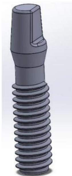
Figure 2. Single thread with Pitch of 0.8 mm
