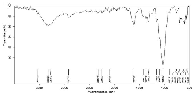
Figure 9. Spectra of water hyacinth stems impregnated (time 3 h) with modified polystyrene
