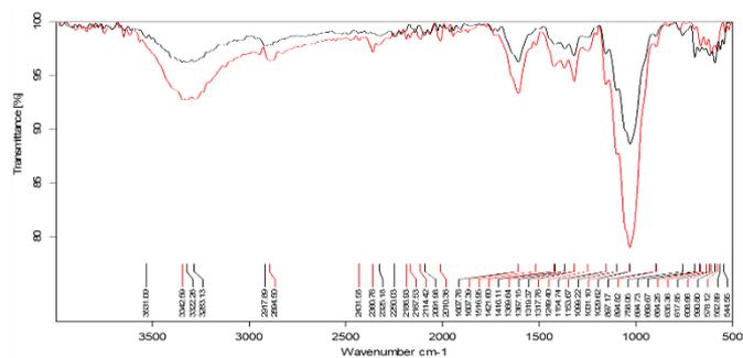
Figure 10. Comparative spectra of FT-IR results of water hyacinth stems and after impregnation (3 h)
