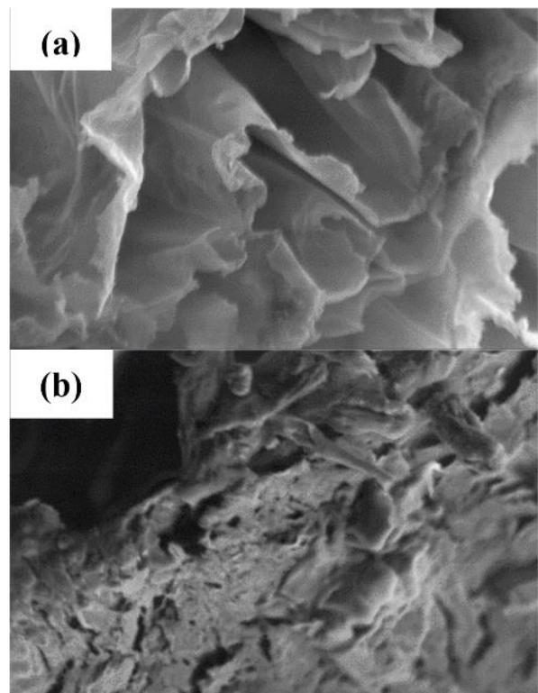
Figure 6. SEM images of water hyacinth stems (inside) before (a) and after (b) impregnation with 4000x magnification
