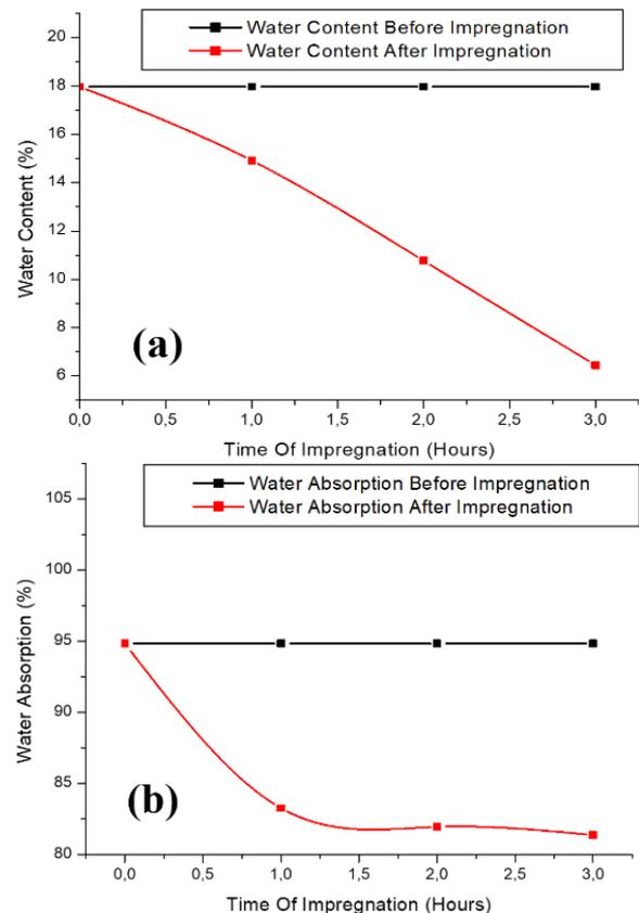
**Figure 3.** Graphs of (a) water content, and (b) water absorption capacity of water hyacinth stems
