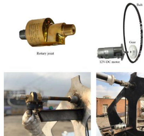
Figure 17. Left: the absorber tube's rotary joint and Right: the DC motor that turns the absorber tube [42]
