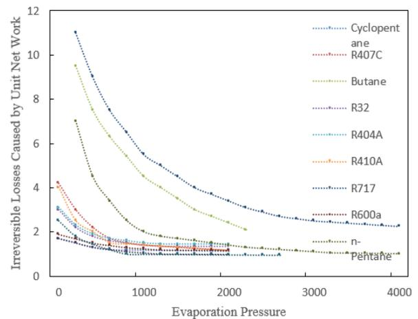
Figure 9. Irreversible losses caused by unit net work
