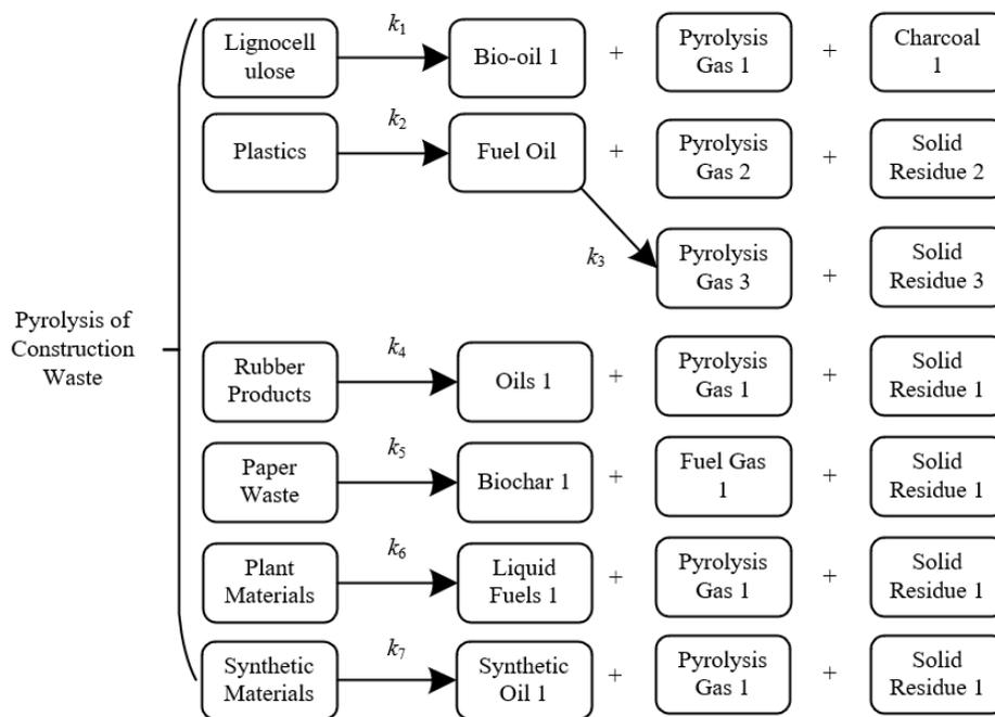
Figure 1. Types of construction waste and products generated by pyrolysis
