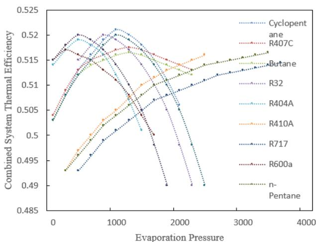
**Figure 10.** Combined system thermal efficiency
