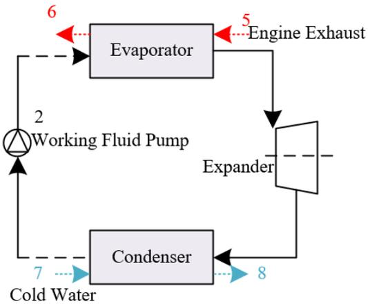
**Figure 3.** Principle of the Rankine cycle
