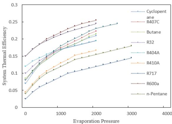
Figure 6. System thermal efficiency
