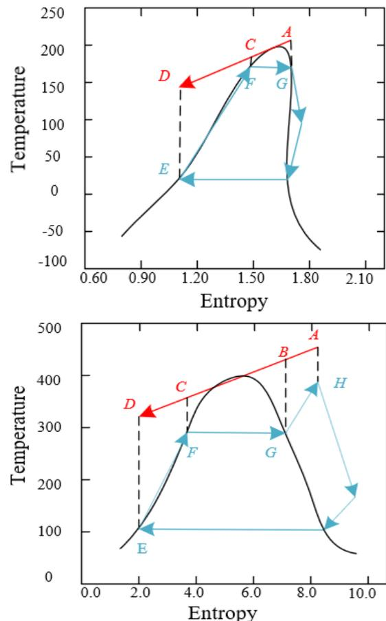
**Figure 4.** Temperature-entropy diagram of subcritical saturated cycle and subcritical superheated cycle
