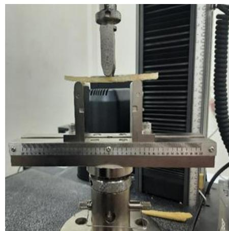
**Figure 4.** Three-point bending test
