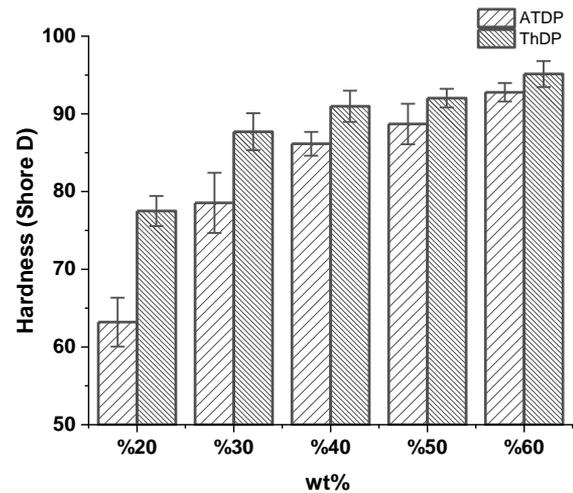
**Figure 10.** Effect of PR weight ratio on the Hardness of EPS/PR hybrid matrix
