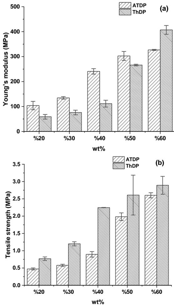
**Figure 7.** Effect of polyester weight ratio on (a) the Young's modulus and (b) the tensile strength of the EPS/PR hybrid matrix
