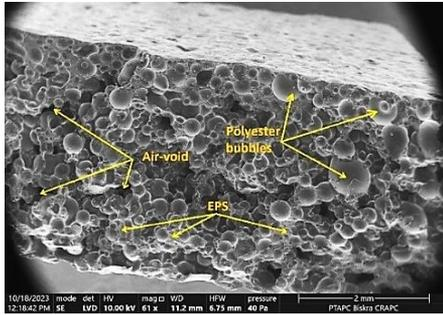
**Figure 11.** Scanning electron microscopy (SEM) image showing the structure of EPS/PR hybrid matrix with 50 wt% of PR
