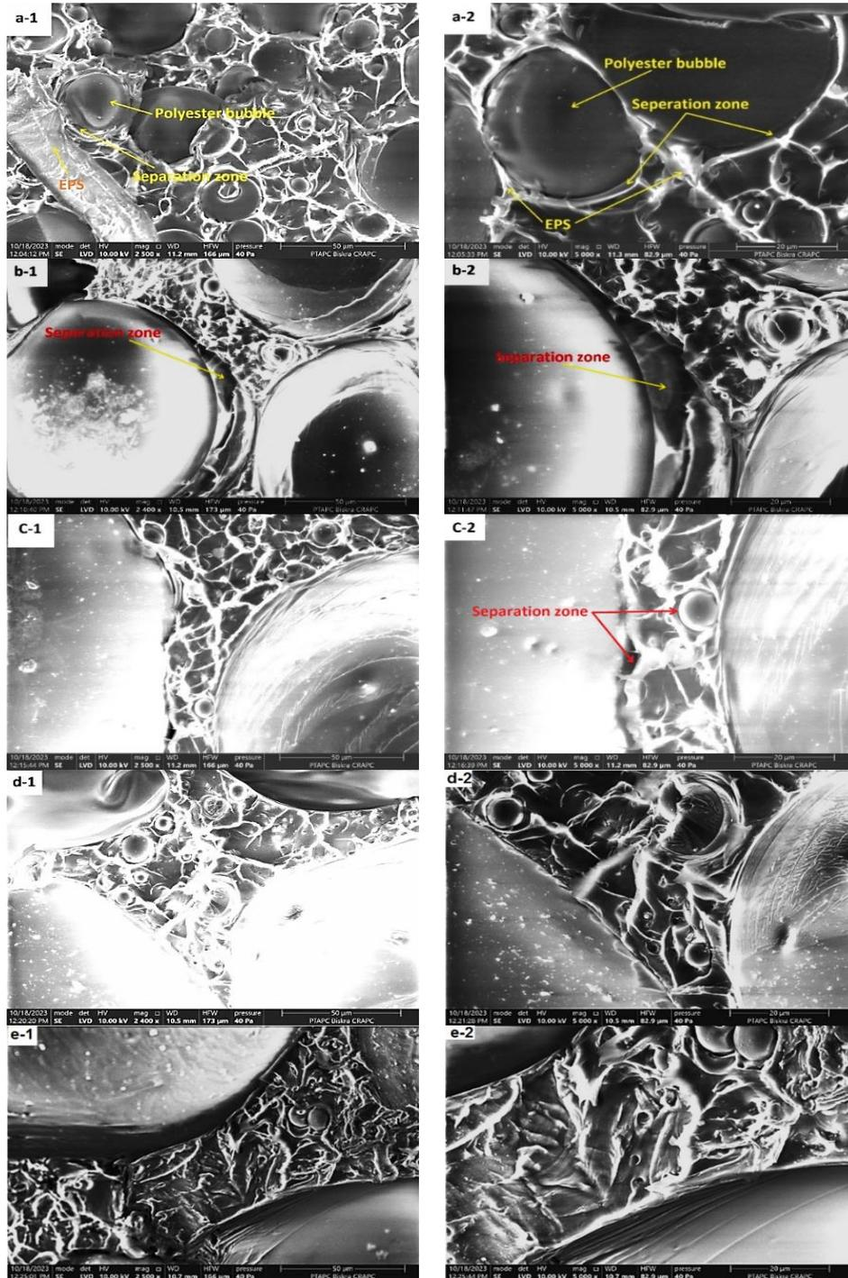
**Figure 12.** SEM figures of EPS/PR hybrid matrix with different weight proportions of PR
