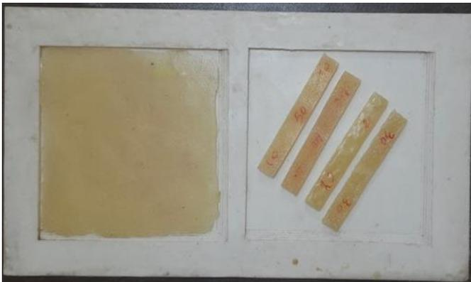
**Figure 2.** The bending test specimens
