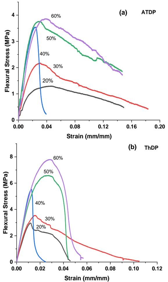
**Figure 8.** Stress-strain type curves of the EPS/PR hybrid matrix obtained from bending tests using (a) ADTP and (b) ThDP processes
