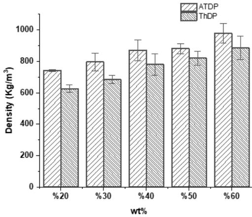
Figure 5. The bulk density of the EPS/PR hybrid matrix
