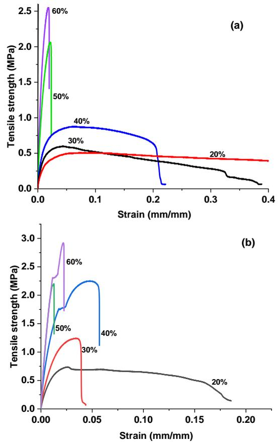
Figure 6. Stress-strain type curves of the EPS/PR hybrid matrix tensile tests: (a) Ambient temperature drying process (ATDP) (b) Thermal drying process (ThDP) at 60°C
