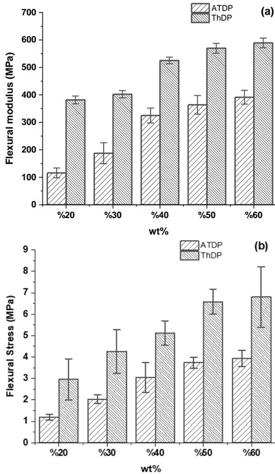
**Figure 9.** Effect of weight ratio of polyester (PR) on (a) the flexural modulus and (b) the flexural strength of the EPS/PR hybrid matrix
