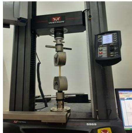
**Figure 3.** Tensile test
