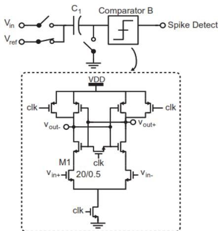
**Figure 4.** Schematic spike detector circuit with spike output in the technology of 180 nm
