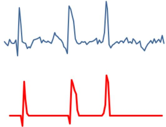
**Figure 5.** The blue diagram is the stored signal and the red diagram shows the output of the Spike detection circuit, which are Spikes according to the use of the capacitor switches
