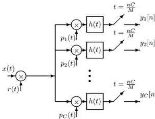
Figure 7. The system used to compress the analog signal using the compression sampling technique
