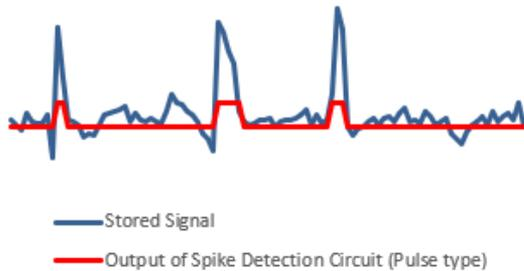
**Figure 3.** The blue diagram shows the stored signal, and the red diagram shows the output of the Spike detection circuit
