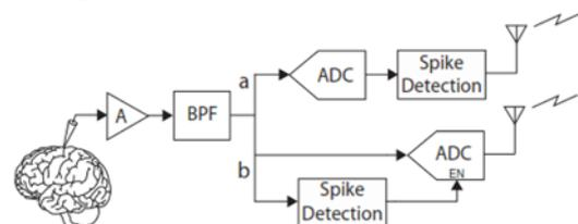
**Figure 2.** The location of the analog and digital processor in the neural signal recording system
