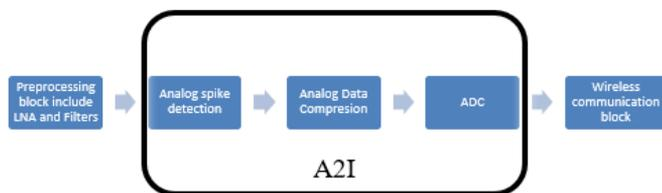
**Figure 9.** Neural signal recording block diagram using spike detection and compressive sampling
