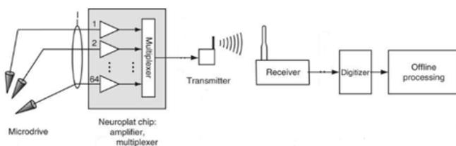
**Figure 1.** Typical multi-channel neural recording system
