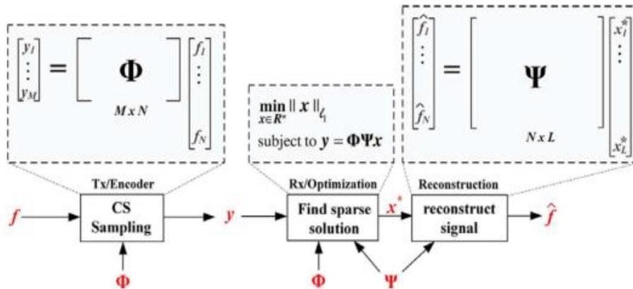
Figure 6. Function of compression sampling technique
