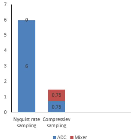
Figure 8. Comparison of power consumption of compressive sampling and sampling at Nyquist rate
