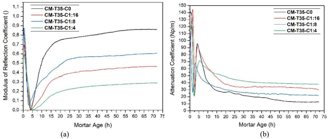
**Figure 7.** Influence of different tested clay dosages on ultrasound parameters evolution during 72h of mortar age, cured at a temperature of 35°C: (a) Evolution of modulus of reflection coefficient; (b) Evolution of attenuation coefficient
