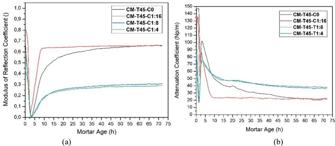
**Figure 8.** Influence of different tested clay dosages on ultrasound parameters evolution during 72h of mortar age, cured at a temperature of 45°C: (a) Evolution of modulus of reflection coefficient; (b) Evolution of attenuation coefficient
