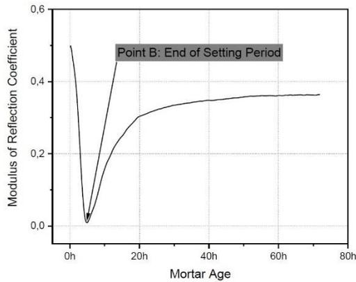
**Figure 2.** Position of characteristic point B on the time evolution curve of modulus of reflection coefficient
