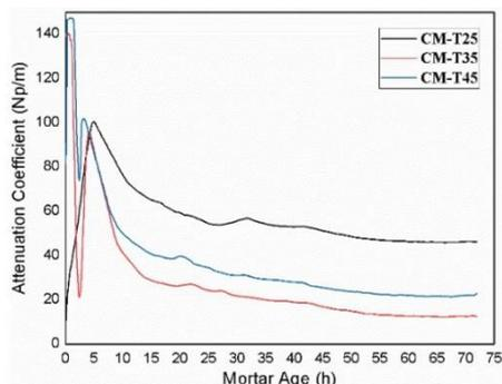
**Figure 5.** Influence of different curing temperatures (25°C, 35°C and 45°C) on attenuation coefficient evolution during 72 h of mortar age
