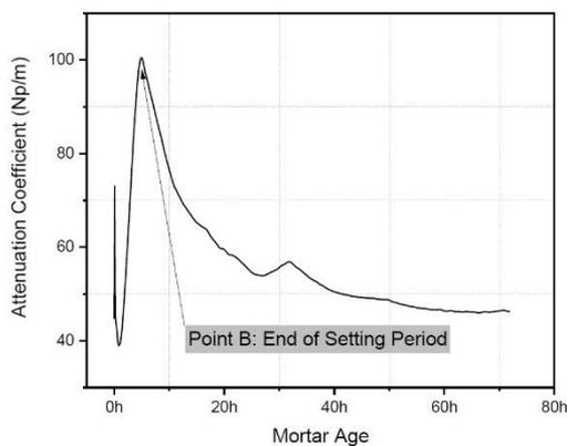
**Figure 3.** Position of characteristic point B on the time evolution curve of attenuation coefficient
