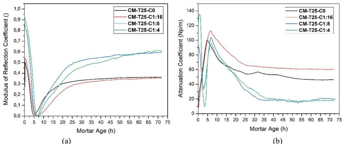
**Figure 6.** Influence of different tested clay dosages on ultrasound parameters evolution during 72h of mortar age, cured at a temperature of 25°C: (a) Evolution of Modulus of reflection coefficient; (b) Evolution of Attenuation Coefficient
