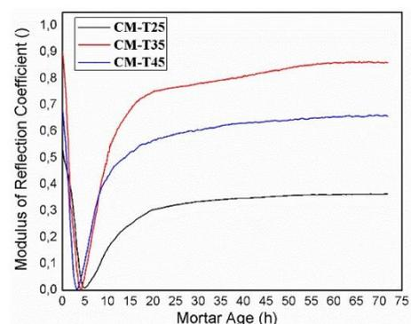
**Figure 4.** Influence of different curing temperatures (25°C, 35°C and 45°C) on modulus of reflection coefficient evolution during 72 h of mortar age
