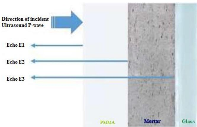
**Figure 1.** Container media and pulse echoes generated from boundaries
