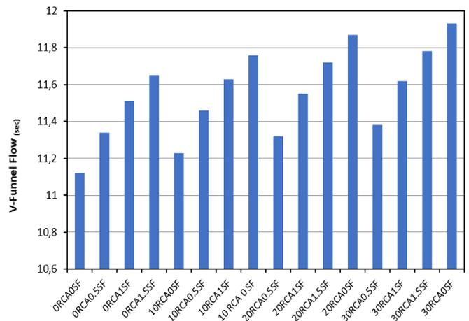
Figure 12. Test results of SCGC mixture (V-funnel test)
