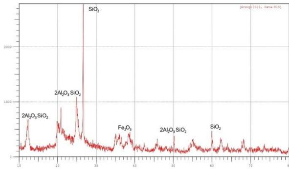
Figure 2. XRD spectra of metakaolin
