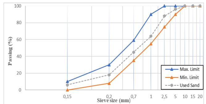
Figure 5. Grading of fine aggregate
