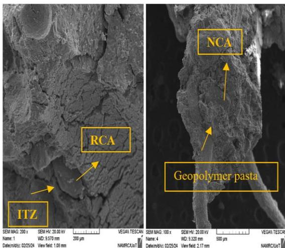
Figure 15. SEM image of geopolymer concrete incorporating: a) recycled coarse aggregate and b) normal aggregate
