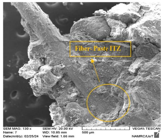
Figure 17. SEM micrograph of geopolymer concrete containing SF
