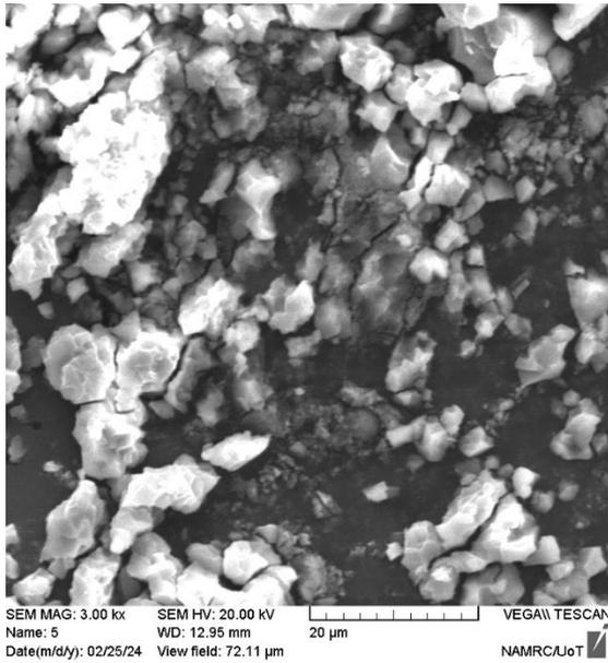
Figure 3. Scanning electron microscopy (SEM) of metakaolin
