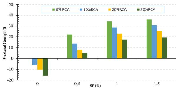
Figure 18. Flexural strength results
