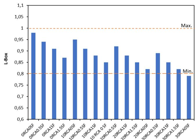
Figure 13. Test results of SCGC mixture (L-Box)
