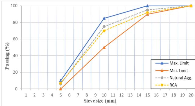
Figure 8. Grading of NCA and RCA
