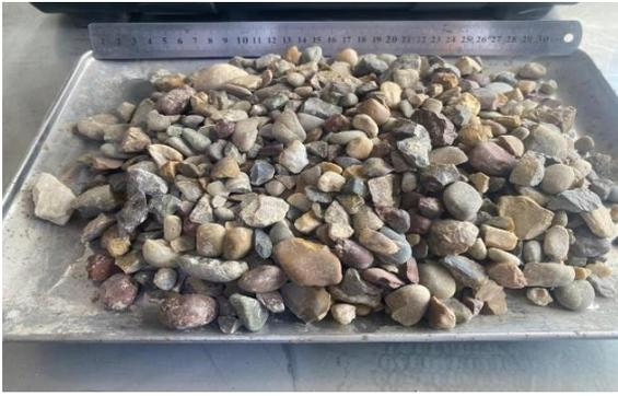
Figure 7. Coarse natural aggregate
