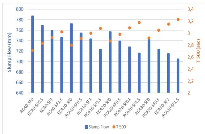
Figure 11. Slump flow and T<sub>500</sub> results of SCGC mixture
