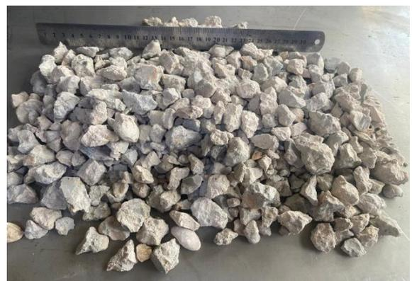
Figure 6. Coarse recycled aggregate
