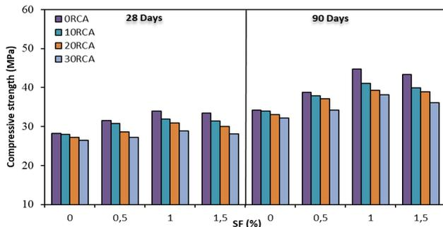
Figure 14. Compressive strength results
