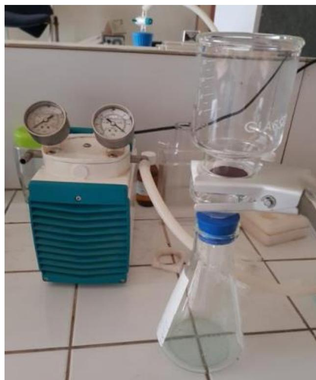
**Figure 2.** Vacuum filtration assembly
