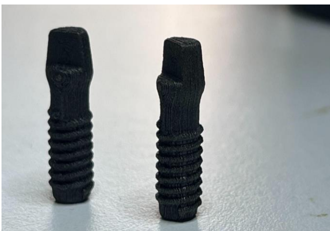
Figure 6. 3D printed implant with 1.2mm thread pitch
