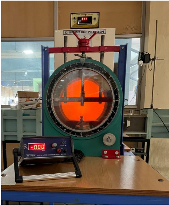
Figure 7. Photoelasticity experimental setup
