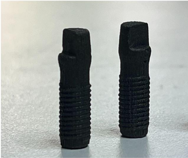
Figure 4. 3D printed implant with 0.8mm thread pitch
