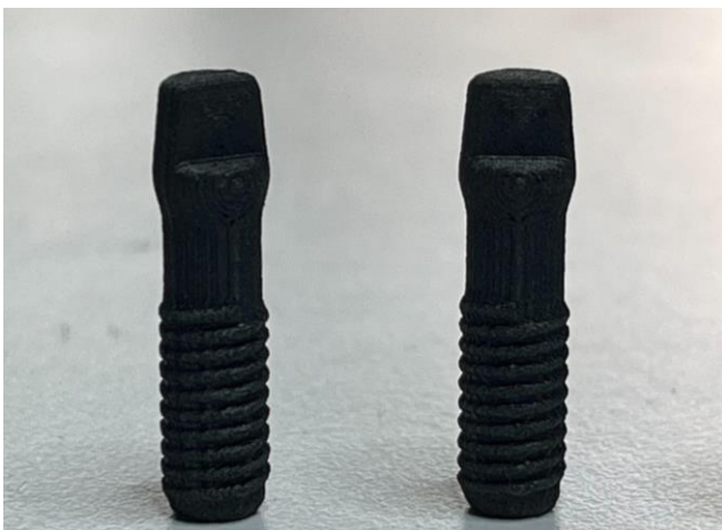
Figure 5. 3D printed implant with 1mm thread pitch
