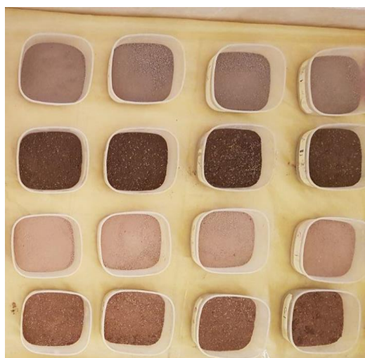
Figure 1. Soil samples after contamination with lead
