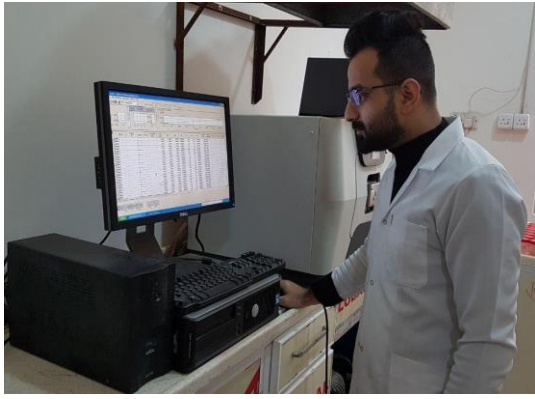
Figure 2. Using atomic absorption spectrometry to estimate lead removed from soil samples
