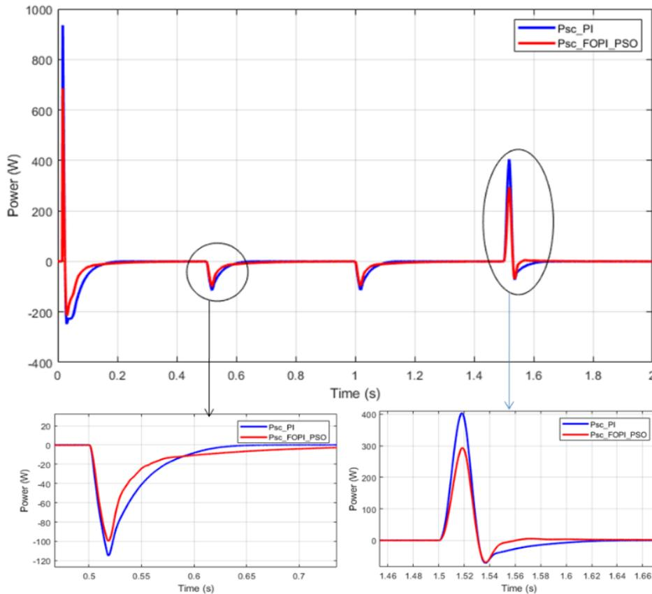
Figure 12. Power responses of SCs for variable solar irradiance with PI and FOPI-PSO controllers
