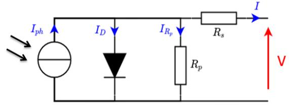
**Figure 2.** Photovoltaic equivalent circuit model
