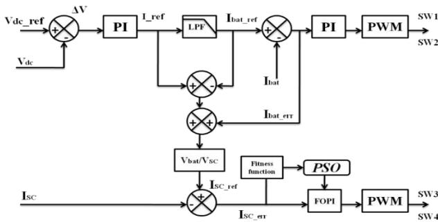
**Figure 9.** Proposed FOPI-PSO hybrid energy storage system control scheme
