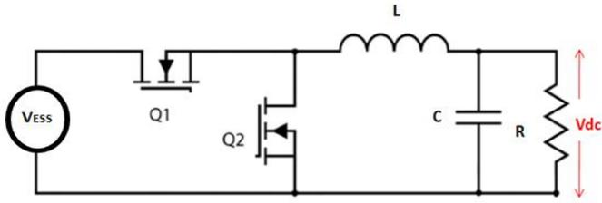
Figure 3. Buck-BOOST DC/DC converter circuit model
