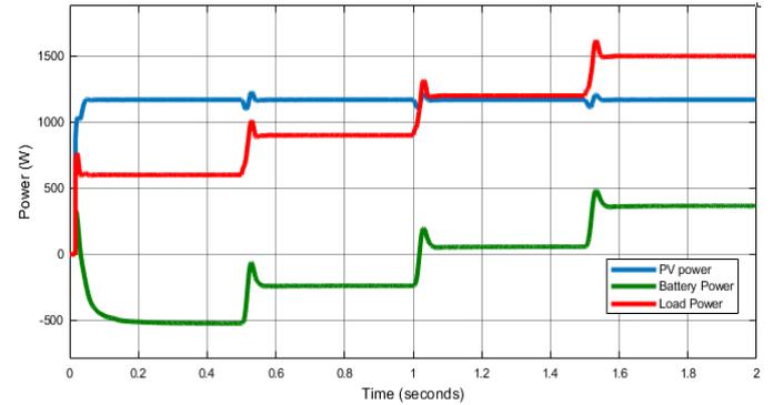
**Figure 13.** Power responses of PV batteries and load with variable load
