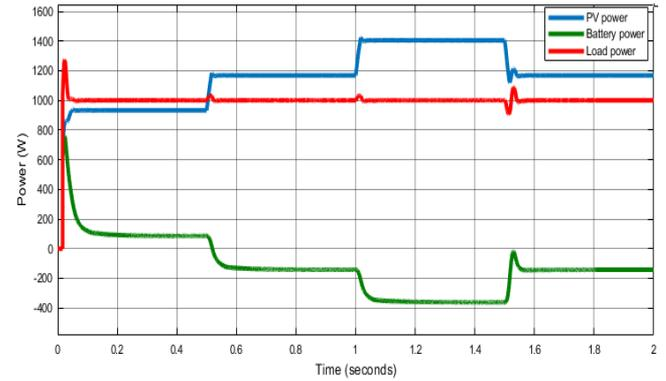
Figure 11. Power responses of PV, batteries and load with variable solar irradiance
