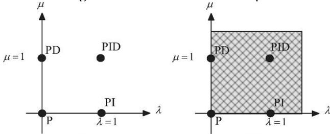
Figure 6. PID controller versus FOPID controller
