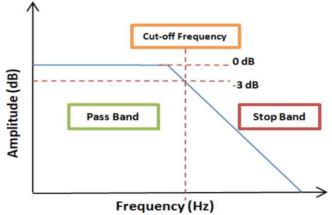
Figure 4. Low pass filter diagram
