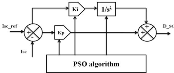
**Figure 8.** Proposed FOPI-PSO controller bloc diagram
