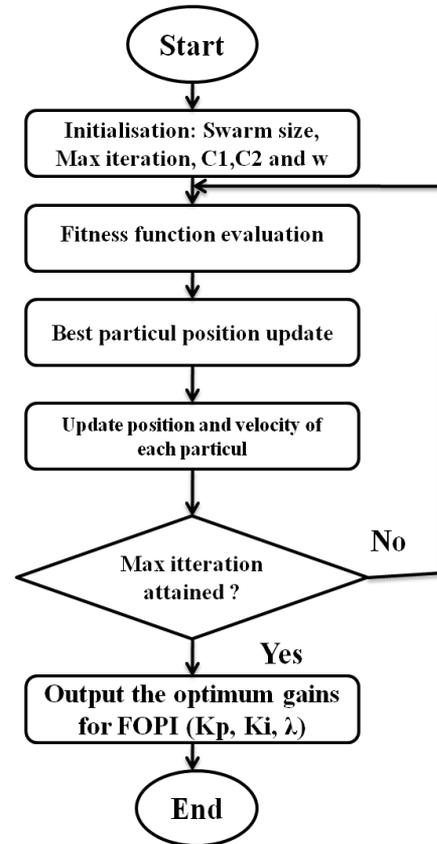
Figure 7. Sequential steps of the Particle Swarm Optimization (PSO) process
