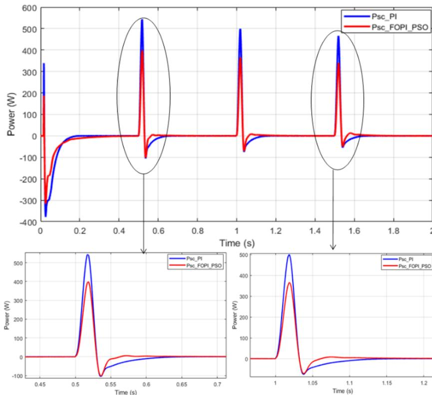
**Figure 14.** Power responses of SCs for variable load with PI and FOPI-PSO controllers
