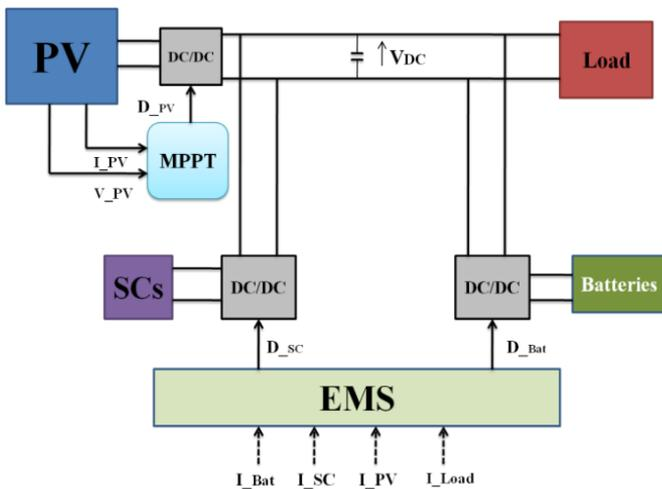
**Figure 1.** Schematic diagram of off-grid PV systems with HESS
