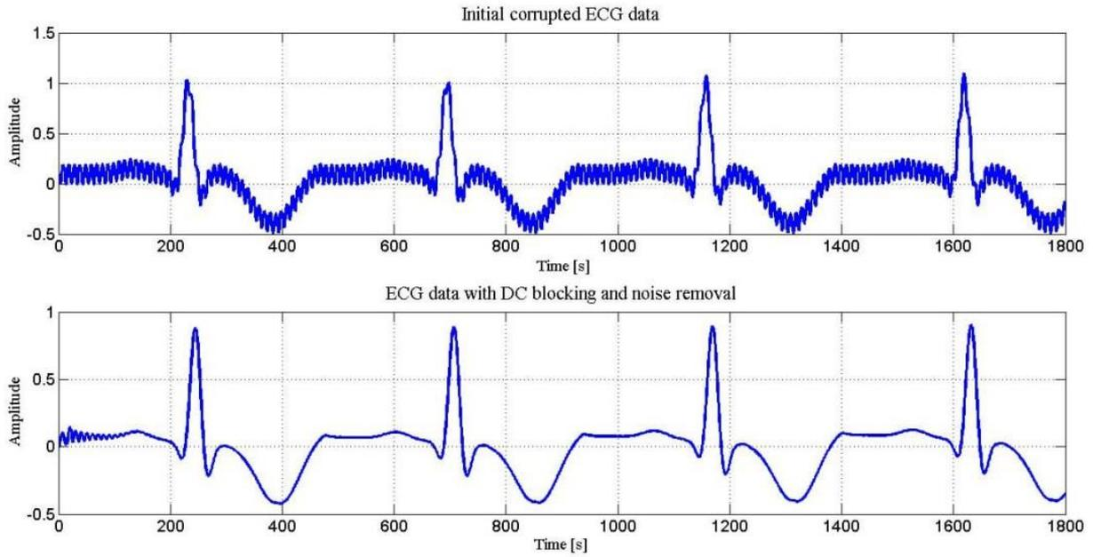
Figure 4. The time domain response of corrupted ECG signal and its filtered output
