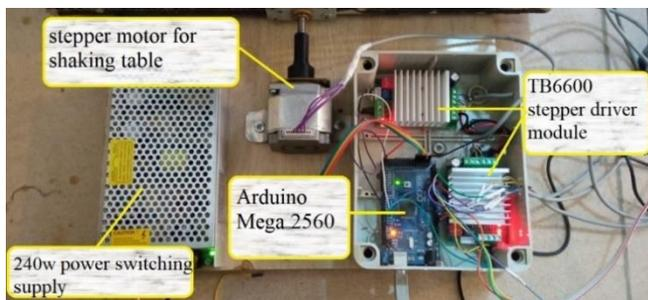
Figure 5. The components of experimental work
