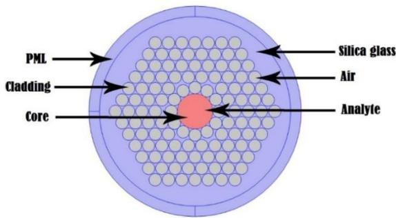
**Figure 1.** Proposed model's internal cross-section
