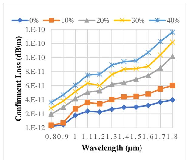
**Figure 7.** Variation of confinement loss versus wavelength for proposed PCF with different concentrations
