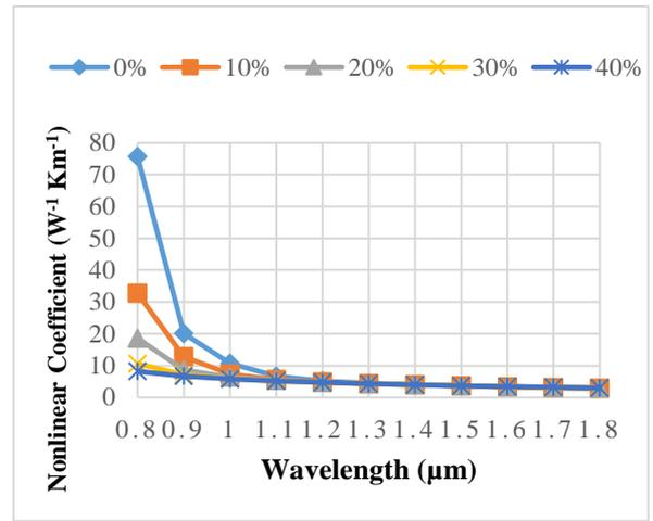
**Figure 9.** Variation of nonlinear coefficients versus wavelength of proposed PCF with different concentrations
