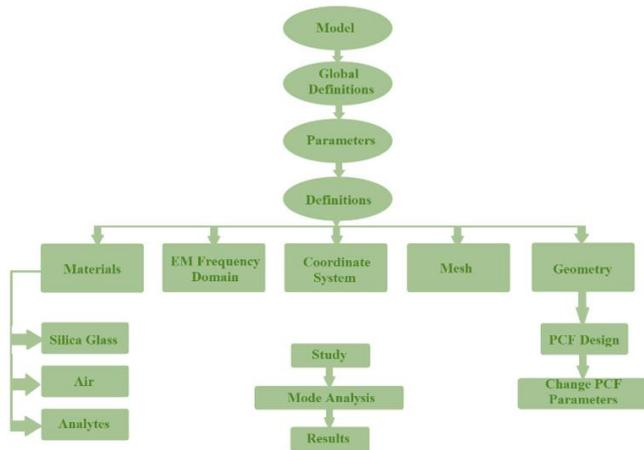
**Figure 2.** The design steps for the PCF structure using COMSOL Multiphysics
