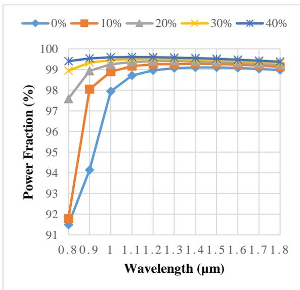
**Figure 5.** Power fraction variation with wavelength for proposed PCF at different concentrations
