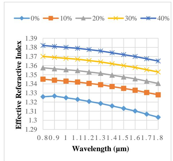
**Figure 4.** Effective refractive index variation with wavelength for proposed PCF at different concentrations
