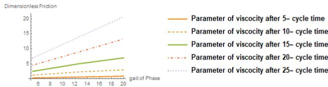
**Figure 8.** Variation of dimensionless Kinematic friction force ( $\zeta^*$ ) with gait phase ( $\omega$ ) for different parametric of viscosity parameters ( $\bar{\mu}$ )
