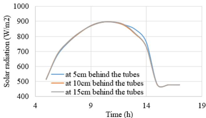
**Figure 8.** Solar radiation gradient by using opacity wall at different space
