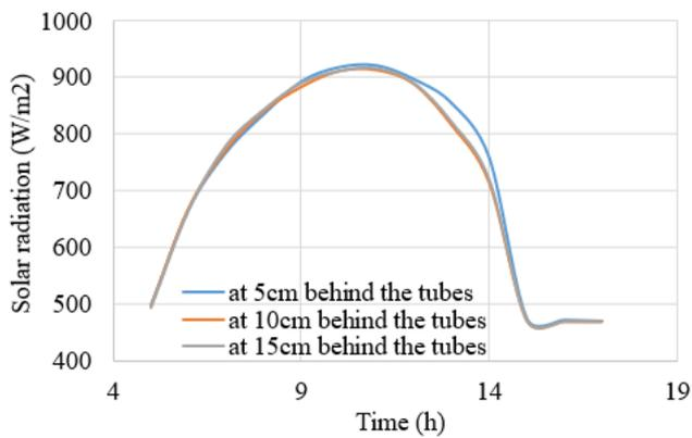
**Figure 5.** Solar radiation gradient by using reflector at different space
