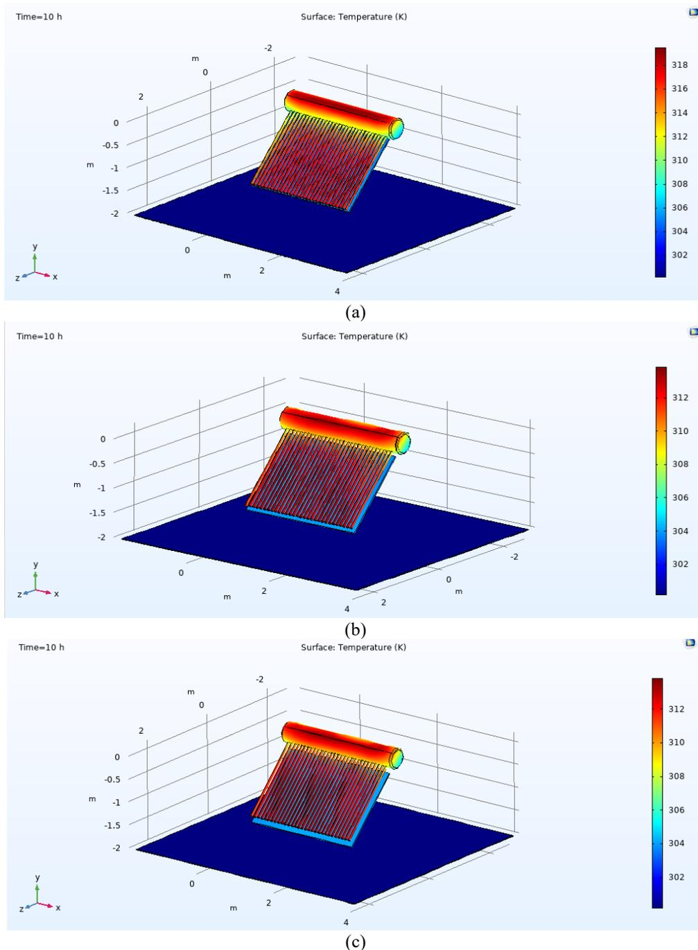
Figure 7. Temperature contour by using opacity wall at different space
