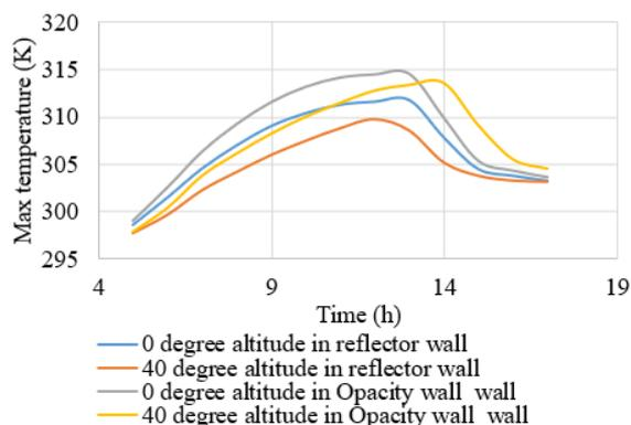
**Figure 9.** Temperature gradient by using opacity wall and reflector wall at different altitude angles
