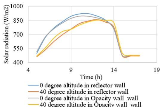
**Figure 10.** Solar radiation gradient by using opacity wall and reflector wall at different altitude angles
