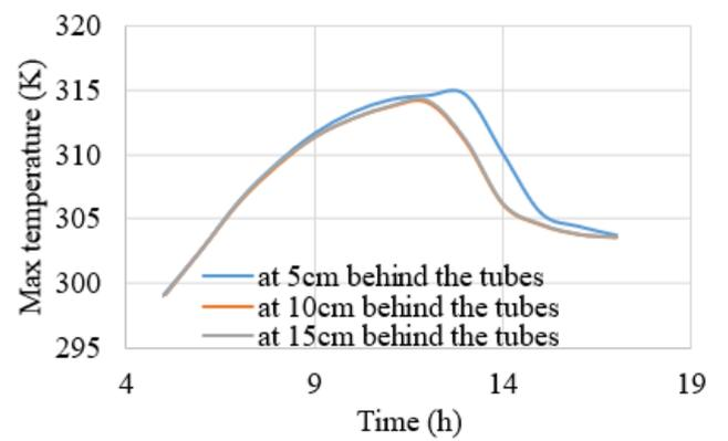
**Figure 6.** Temperature gradient by using opacity wall at different space
