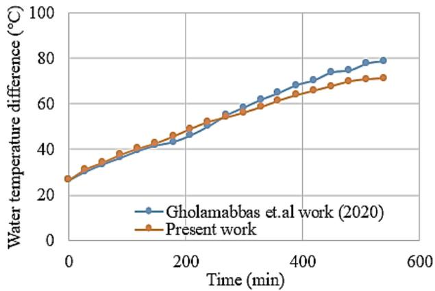
**Figure 11.** The water temperature difference comparison of the numerical and the previous studies
