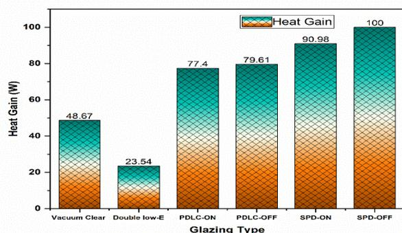
Figure 7. Heat gained by the glass per unit
