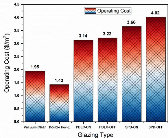
Figure 8. Operating cost of the glass per unit area
