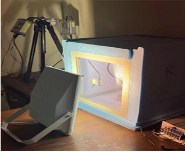
**Figure 3.** Experimental setup with 150 W Osram metal halide lamp
