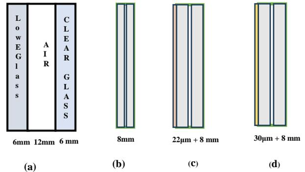
**Figure 2.** Various glass systems studied with its thickness
