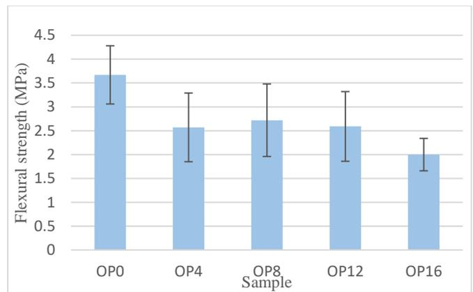
**Figure 13.** Flexural strength for different samples of mixtures
