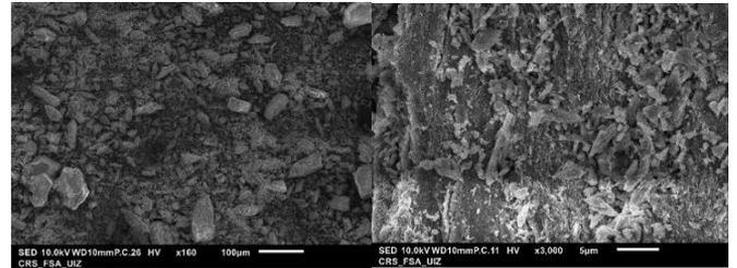
**Figure 4.** Microstructure of gypsum
