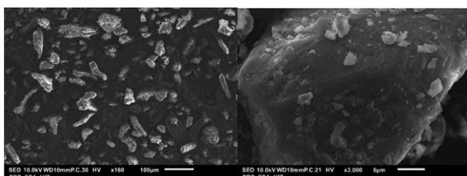
**Figure 3.** Microstructure of olive pomace powder
