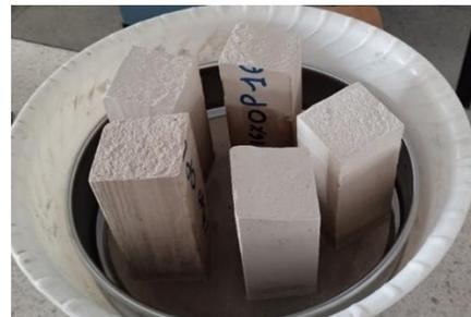
Figure 9. Water absorption by capillarity
