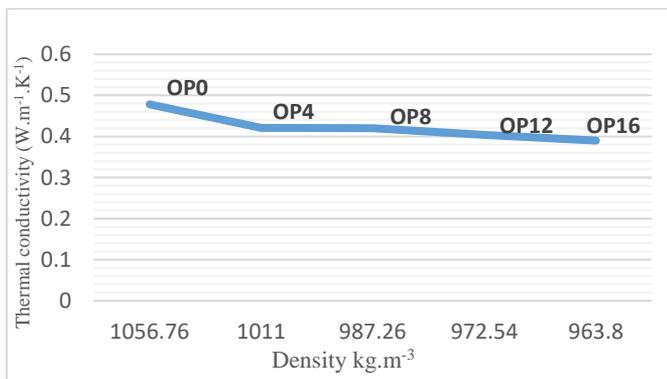
**Figure 12.** Thermal conductivity as a function of density of different composites
