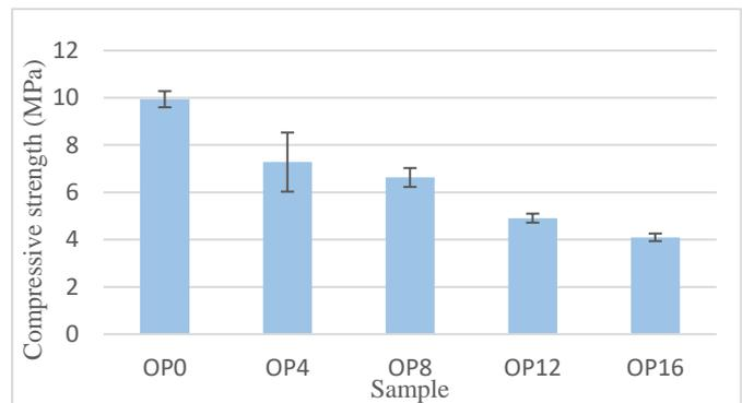
**Figure 14.** Compressive strength for different samples of mixtures
