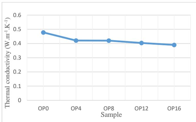
**Figure 11.** Thermal conductivity as a function of OP percentage
