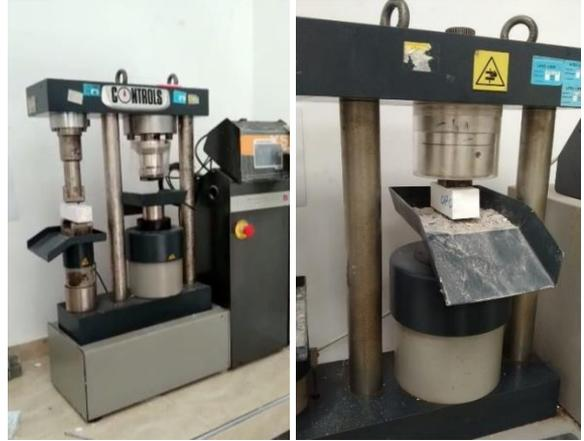
Figure 8. Compression and flexural test
