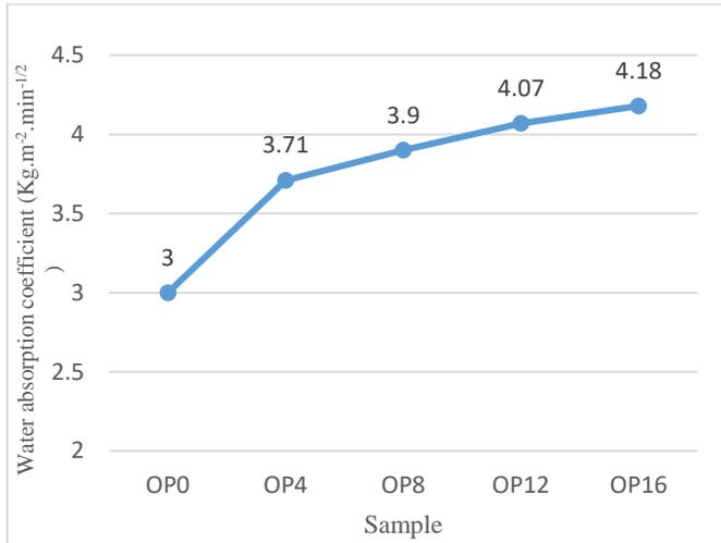
**Figure 15.** Water absorption coefficient as a function of the percentage of OP in the matrix
