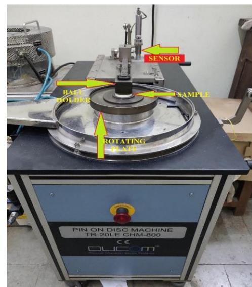
**Figure 2.** Tribometer used for the wear test (ball on disc)
