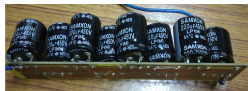
Figure 3. Capacitor Bank hardware model
