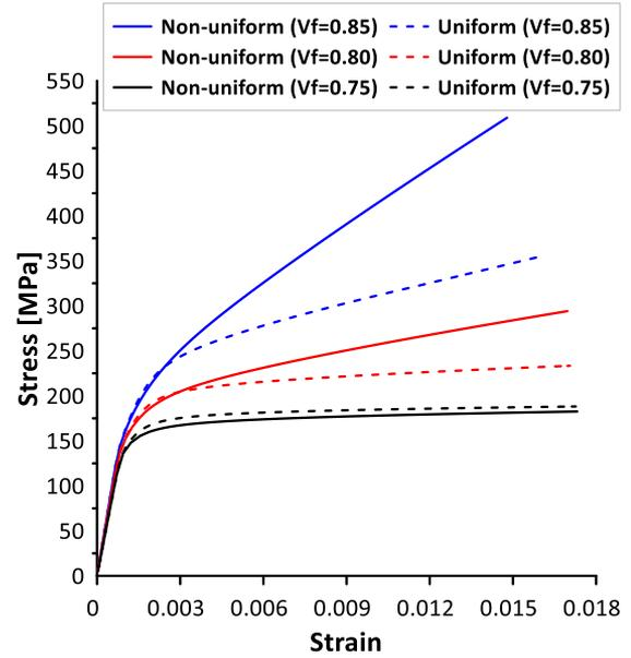
Figure 7. Comparison of obtained stress-strain curves of composites with two different platelet shapes, and three different volume fractions
