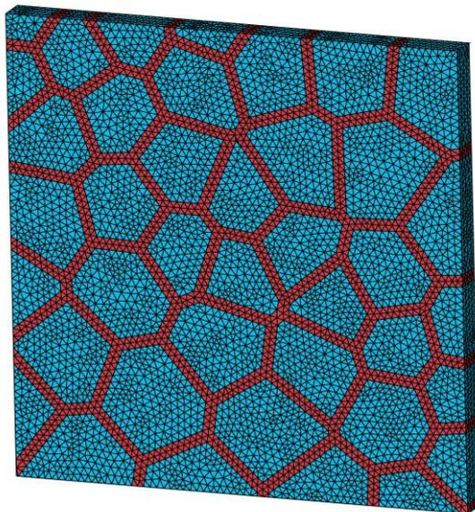
Figure 6. 3D finite element model of platelet-reinforced composite with sharp corners
