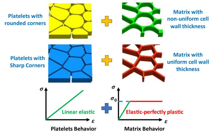
**Figure 3.** 3D models of platelet composites designed with two types of platelet shapes and the mechanical behavior of the constituents
