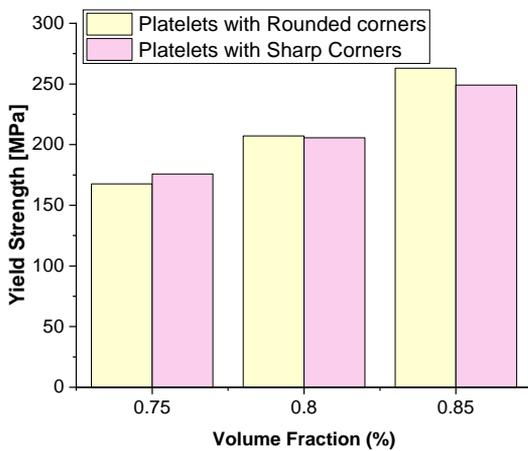
**Figure 9.** Comparison of effective yield strength of the tested composites with two different platelet shapes, and three different volume fractions
