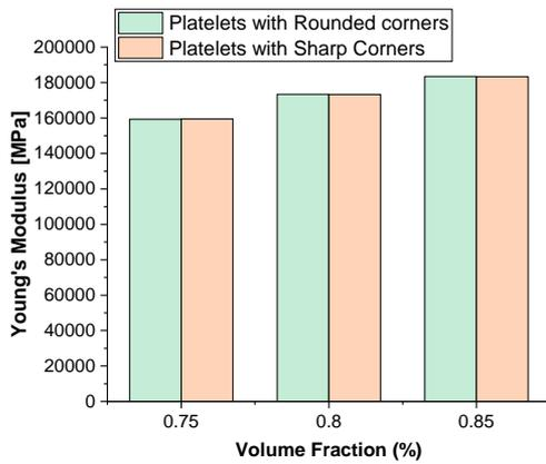
**Figure 8.** Comparison of effective Young's modulus of the tested composites with two different platelet shapes, and three different volume fractions
