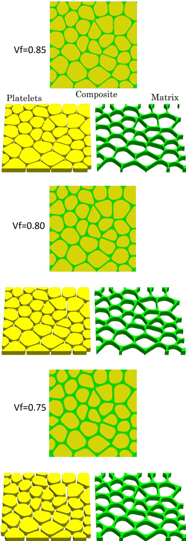
**Figure 2.** 3D Models of designed platelet-reinforced composite with rounded corners for three different volume fractions
