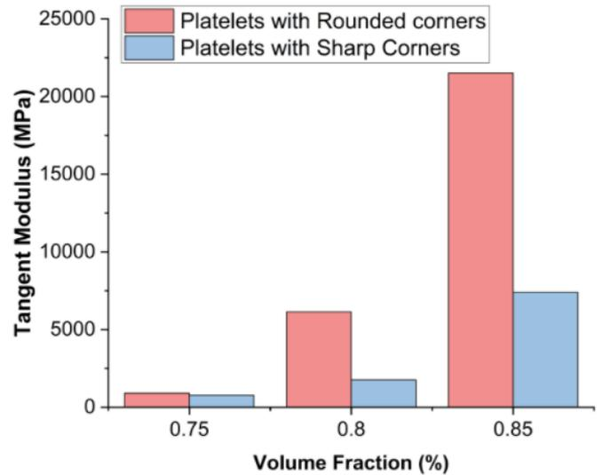
**Figure 10.** Comparison of effective Tangent Modulus of the tested composites with two different platelet shapes, and three different volume fractions
