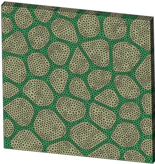
Figure 5. 3D finite element model of platelet-reinforced composite with rounded corners
