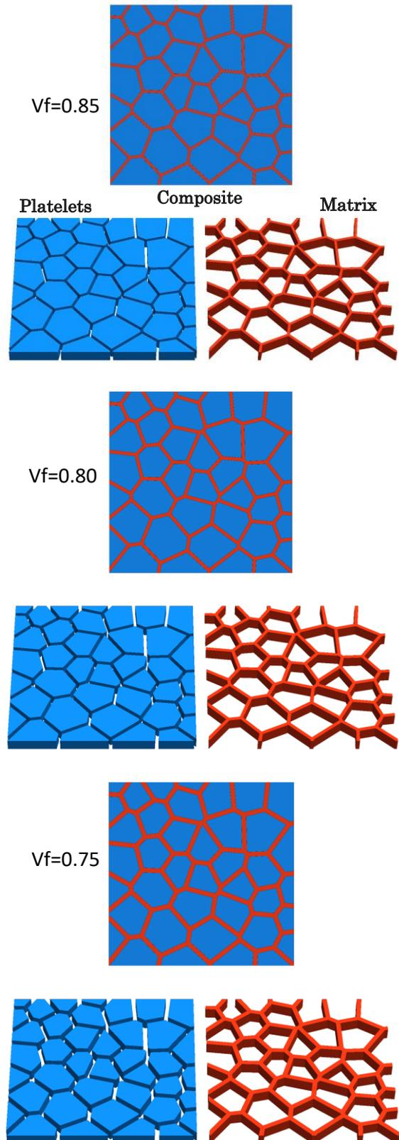
**Figure 1.** 3D Models of designed platelet-reinforced composite with sharp corners for three different volume fractions
