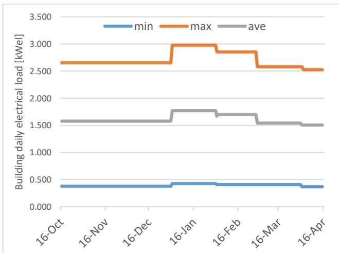
**Figure 4.** Building daily electrical load during the heating period
