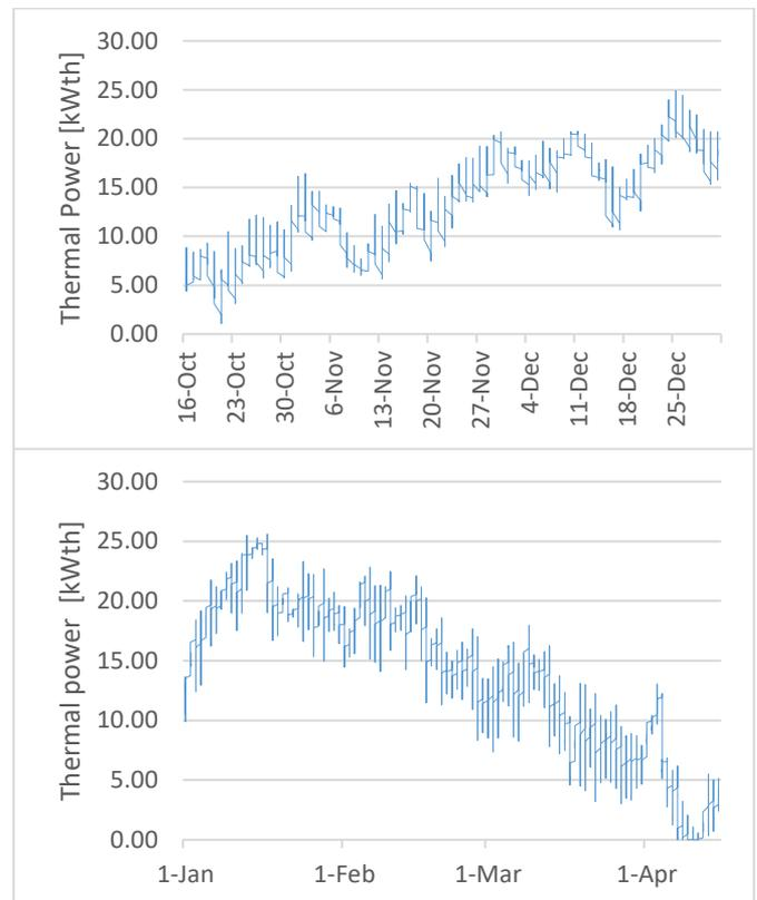
**Figure 3.** Building thermal power demand during the heating period
