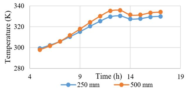
**Figure 6.** Temperature gradient by using mirrors at different mirrors wall width
