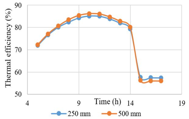
**Figure 9.** Thermal efficiency gradient by using mirrors at different mirrors wall width
