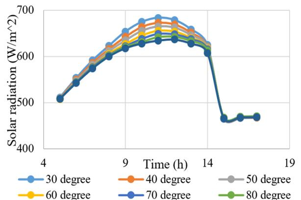
**Figure 4.** Solar radiation gradient by using mirror at different angle between mirror wall and vacuum pipe
