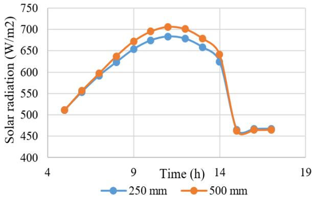
**Figure 7.** Solar radiation gradient by using mirrors at different mirrors wall width
