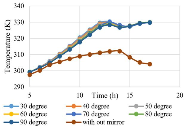
**Figure 3.** Temperature gradient by using mirror at different angle between mirror wall and vacuum pipe
