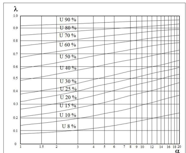
Figure 6. Determination U (%) based parameter  $\alpha$  &  $\lambda$
