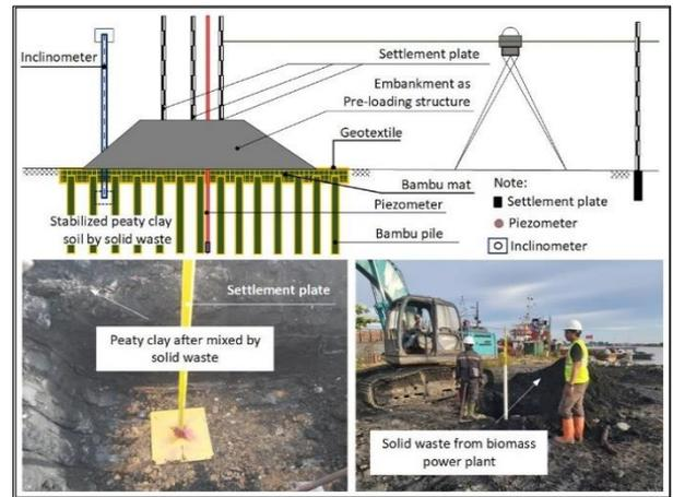
Figure 5. Measurement using the settlement plate device
