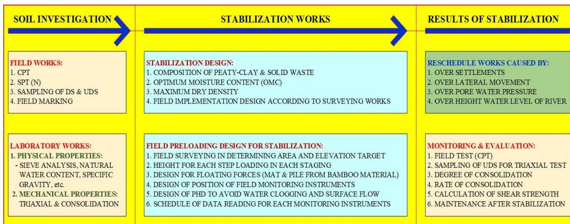
Figure 3. Flow model for peaty clay soil stabilized by solid waste from biomass power plant
