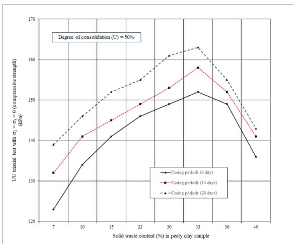
**Figure 7.** Graphic of standard proctor test for peaty clay soil stabilized by various amounts of solid waste versus compressive strength at 0, 14, and 28 days of curing periods
