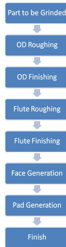
**Figure 6.** Simulation model for CNC
