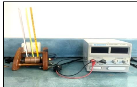
Figure 4. The thermal conductivity test device
