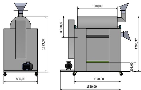
Figure 2. Technical drawing of a biomass energy-based roasting machine (unit: mm)
