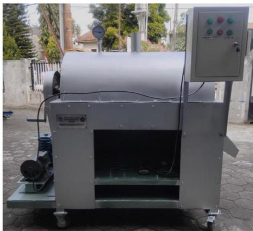
**Figure 3.** Photograph of a biomass energy-based roasting machine
