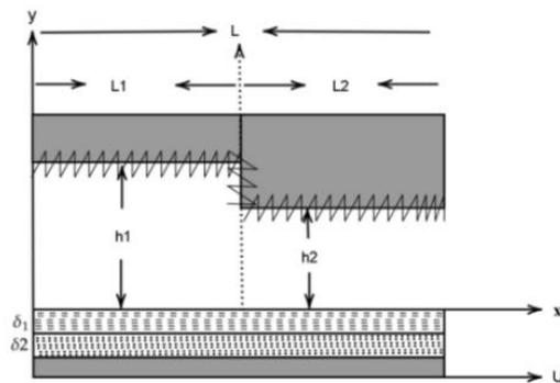
Figure 1. Double porous Rayleighstep slider bearing
