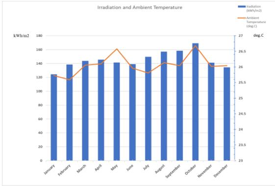
**Figure 4.** Monthly average irradiation and ambient temperature
