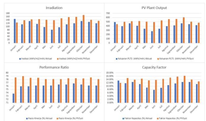
**Figure 7.** Output comparison, PR and CF between actual data and PVsyst simulation
