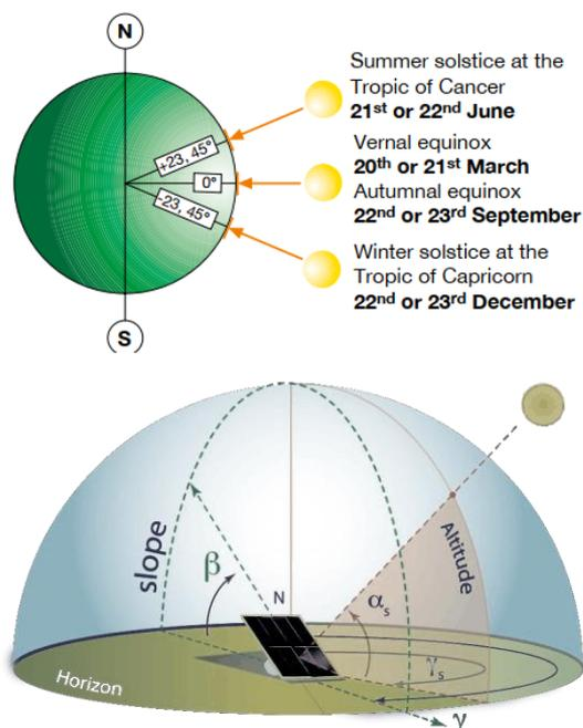
**Figure 8.** Declination, altitude of the sun and its relation to the tilt of the solar module [19]
