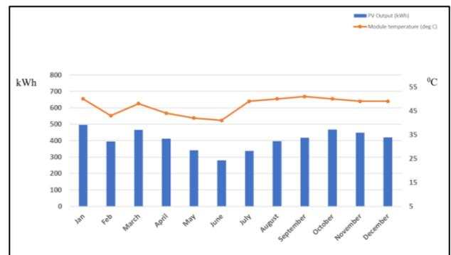
**Figure 6.** Energy output and average module temperature in the PV power plant
