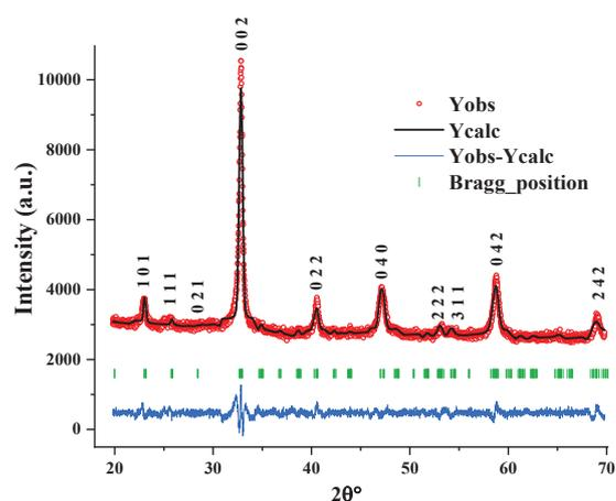
**Figure 3** The profile plot and the crystal structure of Sm<sub>0.6</sub>Sr<sub>0.4</sub>MnO<sub>3</sub>
