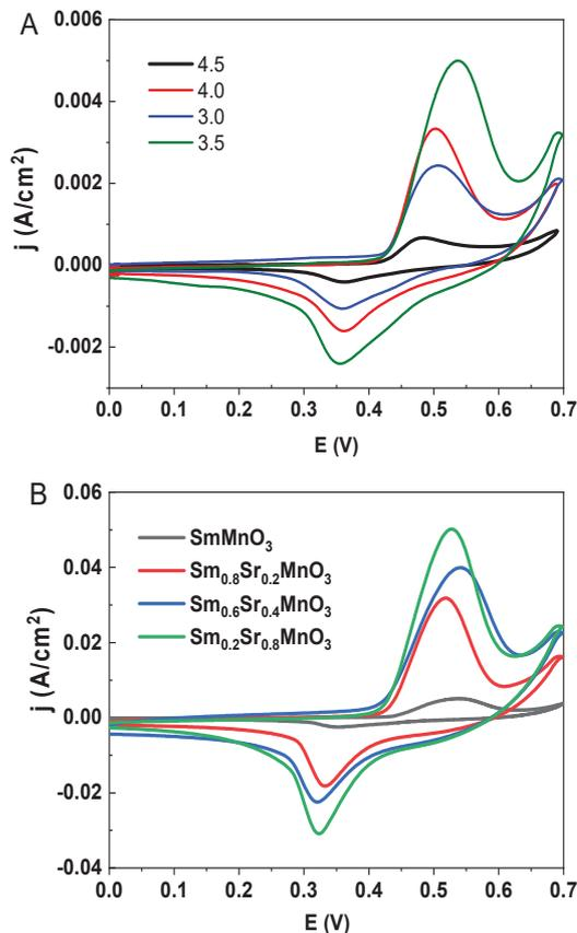
**Figure 4 (A):** Cyclic voltammograms of  $\text{SmMnO}_3$  film electrode at different pH on Ni at  $20 \text{ mV/sec}$  scan rate in 1 M KOH ( $25^\circ\text{C}$ ). **(B)** Cyclic voltammogram of pure and Sr-substituted manganite (pH = 3.5) film electrode on Ni at  $20 \text{ mV/sec}$  scan rate in 1M KOH ( $25^\circ\text{C}$ )
