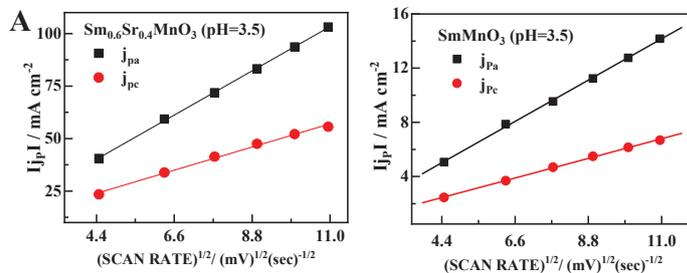
**Figure 5 (A):** Plot of  $|j_p|$  vs  $(\text{scan rate})^{1/2}$  for the oxide film electrodes on Ni in 1M KOH at ( $25^\circ\text{C}$ )
