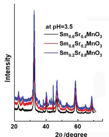
**Figure 2:** XRD powder patterns Sintered at 650°C for 5h
