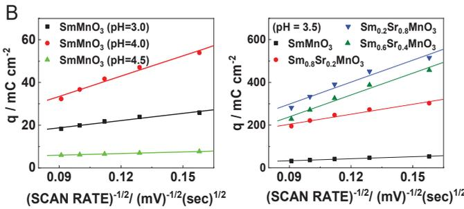
**Figure 5 (B):** Plot of  $q$  vs  $(\text{scan rate})^{-1/2}$  for the oxide film electrodes on Ni in 1M KOH at (25°C)
