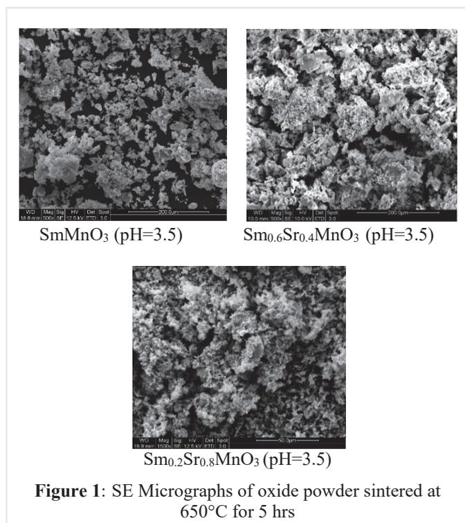
**Figure 1:** SE Micrographs of oxide powder sintered at 650°C for 5 hrs
