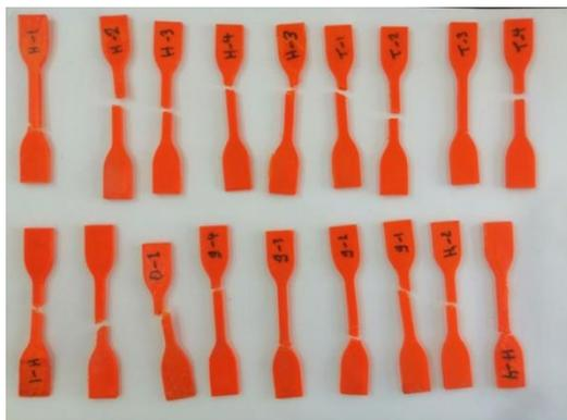
Figure 4. The fractured 3D-printed tensile specimens
