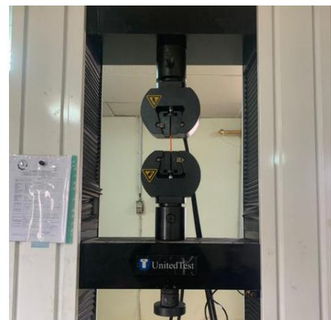
**Figure 2.** Tensile test machine
